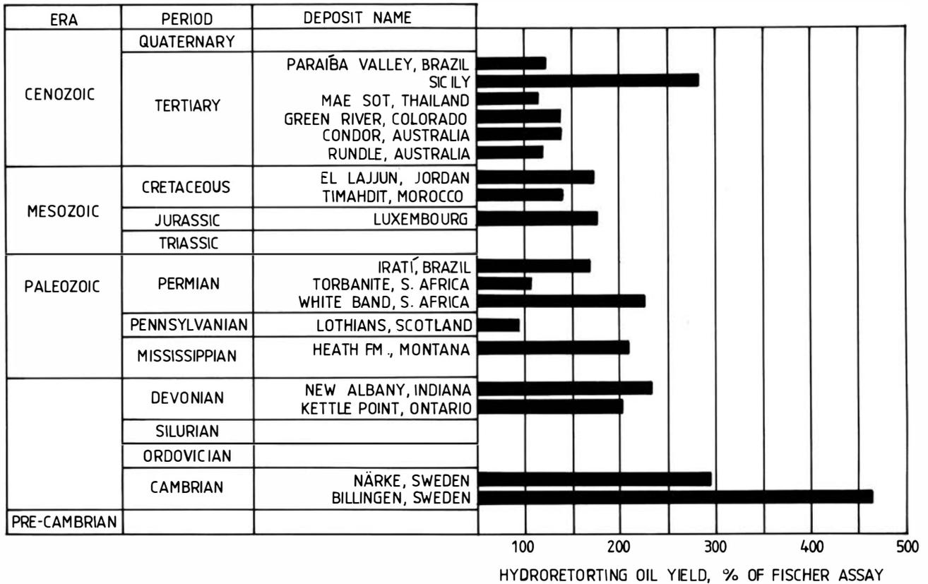
Fig. 24. Hydroretorting assay test results (from Janka & Rex 1984). The Närke and Billingen samples (Fischer assays of 4.4 % and 1.5 %, respectively) yielded 134 litres/tonne and 73 litres/tonne oil, respectively, when retorted in a atmosphere of hydrogen under pressure (7 MPa).
