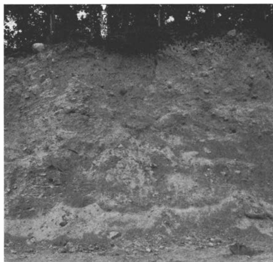
Fig. 28. Section through a short real drumlin S. of Hästveda, N. Skåne. Dense, compact basal till throughout; indistinct foliation in places; boulders mostly towards the top. Ice movement obliquely from the left.
