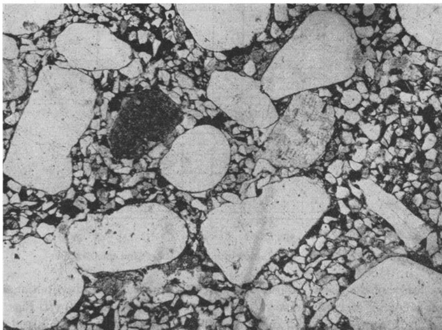
Fig. 15. Ekerö arkose showing polymodal grain-size and roundness distribution. Cement is hematite, the dark large grain is a fine-grained dolerite. Outcrop 18. || nic., 25 ×.
