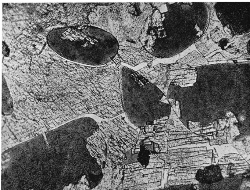
Fig. 58. Grains of glauconite with crystals of siderite and calcite. Below the grain in the middle of the fig. we see the small rest of another grain, the greater part of which is replaced by calcite. Glaucinitic limestone. Ottenby, 8. (Pr. 3000. Pl. 525.) -- 60 \times .
