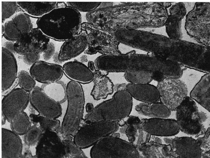
Fig. 41. Glaucinite grains and rounded fragment of fossils and limestone. Cement: clear, colourless chalcedony. Tertiary. Erratic pebble. Ystad. (Pr. 2259. Pl. 623.) — 60 \times .
