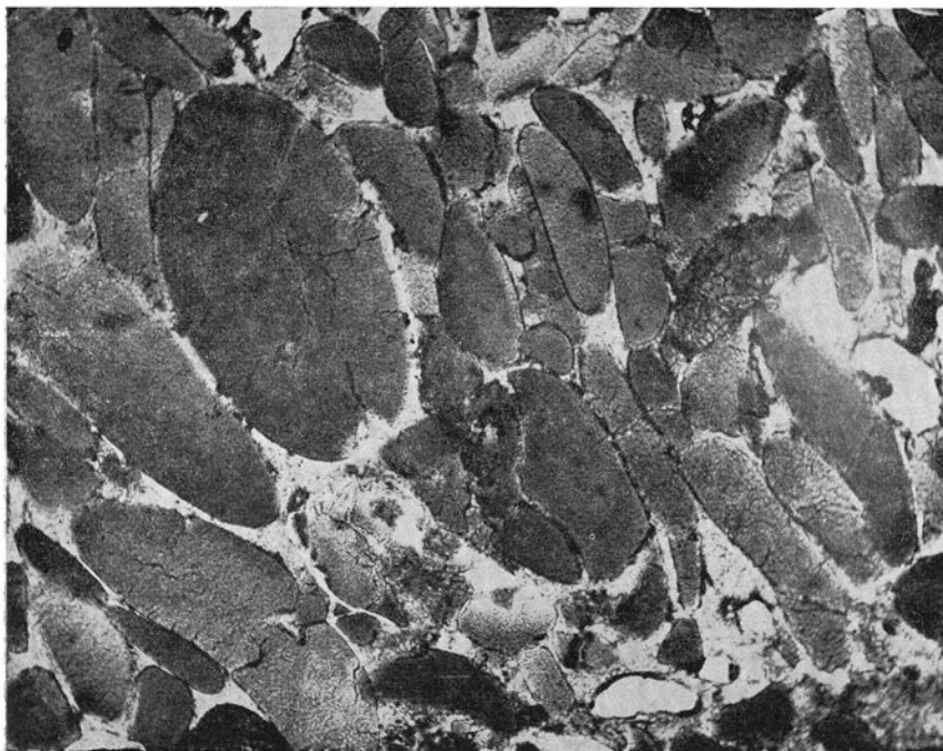
Fig. 53. Tabular grains of glauconite. Glauconite sand. Ceratopyge stage. Pålstorp, Östergötland. (Pr. 3192. Pl. 569 a.) — 60 \times .
