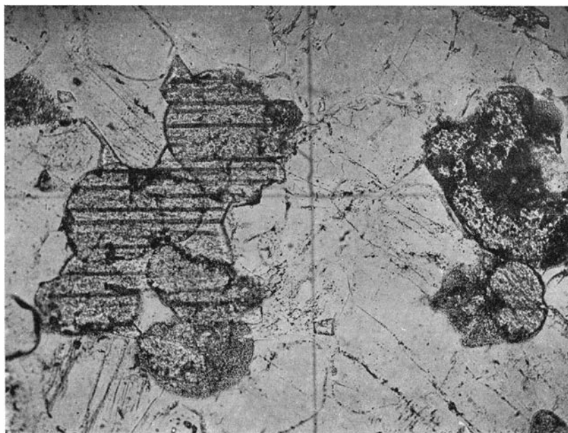
Fig. 60. Grains of glauconite replaced by calcite. Lower Cambrian sandstone, partly calcareous, partly quartzitic. Brantevik, 9 c. (Pr. 3117. Pl. 541.) — 60 \times .
