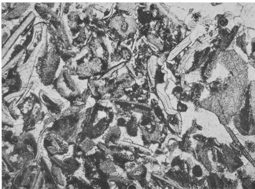
Fig. 160. Fragment limestone with matrix of calcite. *Ludibundus* limestone, Middle Ordovician. Böda harbour, Öland. (Prep. 6619, photo 1350.) — 20 ×.
