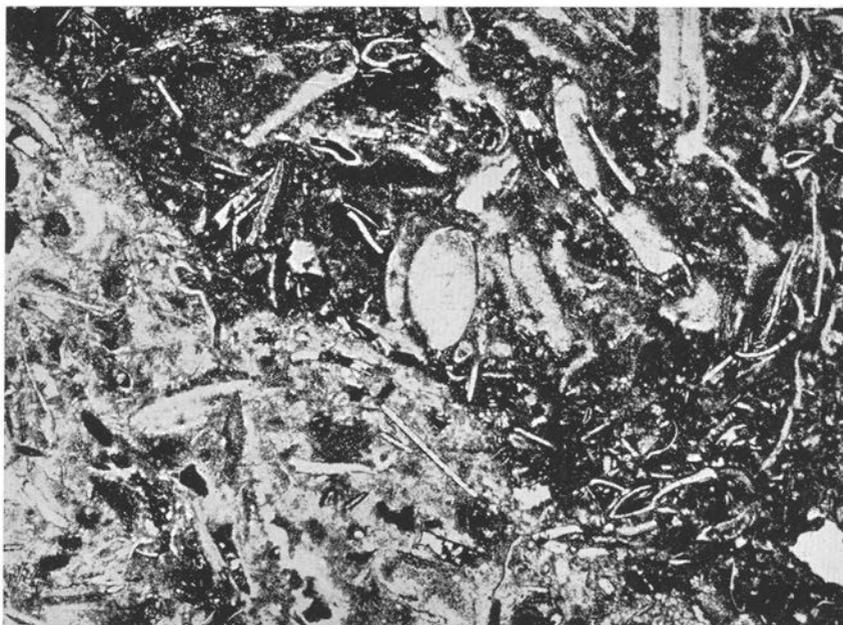
Fig. 127. Gigas limestone. Microcoquina limestone, irregularly pigmented with hematite. Lower Ordovician. Sollerön, Dalarna. (Prep. 7207, photo 1364.) — 20 ×.
