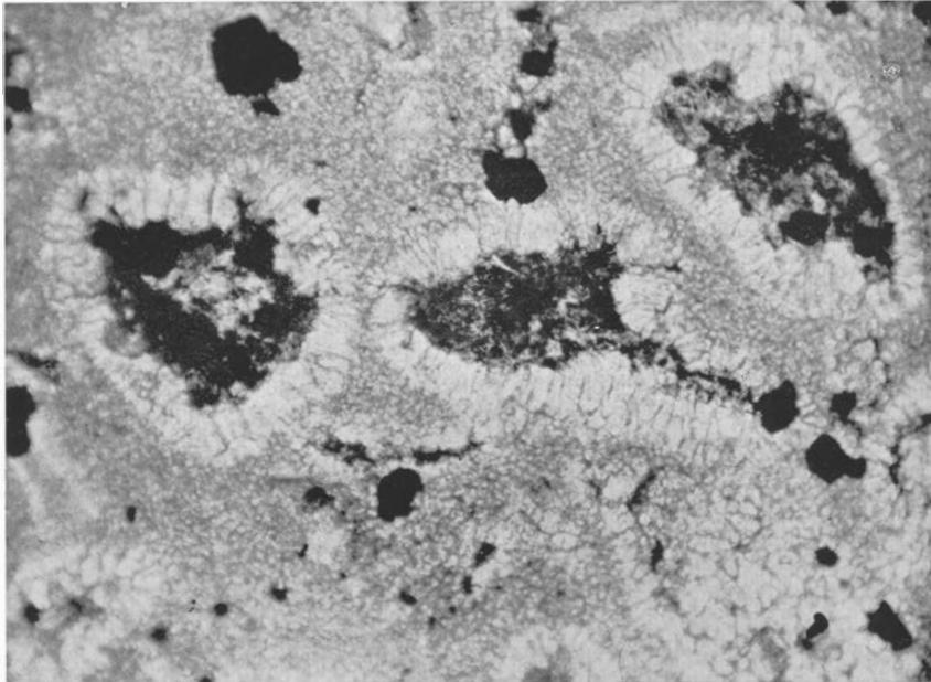
Fig. 31. Crystalline-granular texture. Bitumen pockets with crust of radiated calcite crystals. Ceratopyge limestone. Flagabro, Skåne. (Prep. 6318, photo 1299.) — 60×.
