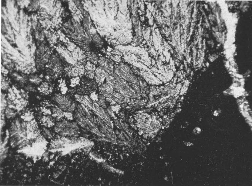
Fig. 54. Fibrous, plume-shaped calcite crystals and microcrystalline, bituminous calcite aggregate. Andrarum limestone, Middle Cambrian. Andrarum, Skåne. (Prep. 6562, photo 1750.) — 20×.
