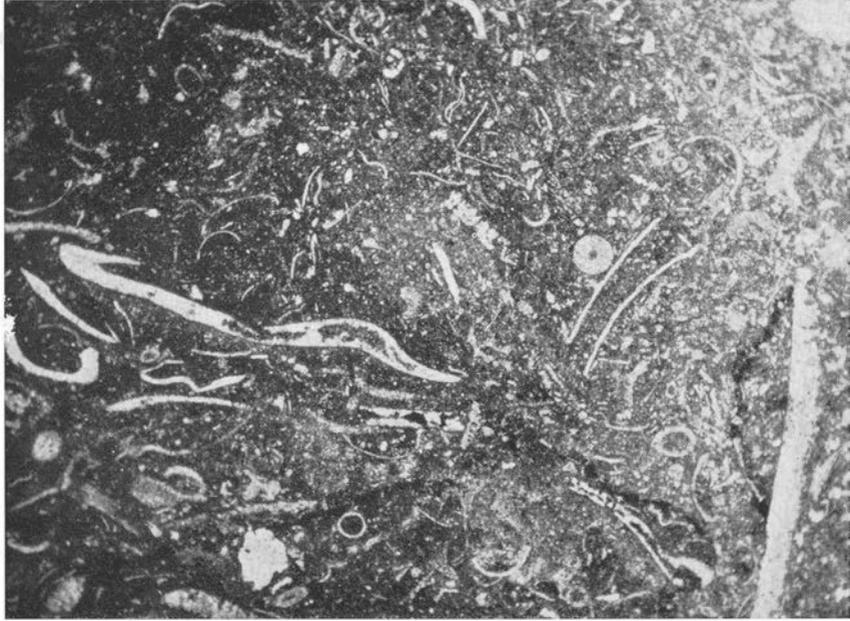
Fig. 133. Platyurus limestone. Microcoquina limestone, strongly pigmented with hematite dust. Lower Ordovician. Loke, Lockne, Jämtland. (Prep. 8773, photo 1619.) — 20×.
