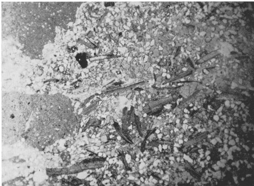
Fig. 44. Arenaceous limestone with phosphorite nodules (left), glauconite grains and phosphatic shell fragments. Lower Cambrian. Andrarum, Skåne. (Prep. 8758, photo 1720.) — 20 ×.
