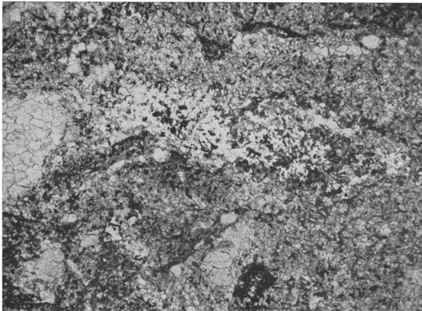
Fig. 181. Microcrystalline limestone, partly silicified (middle part). Dalmanitina limestone, Upper Ordovician. L. Lycke, Billingen, Västergötland. (Prep. 8809, photo 1600.) — 20×.
