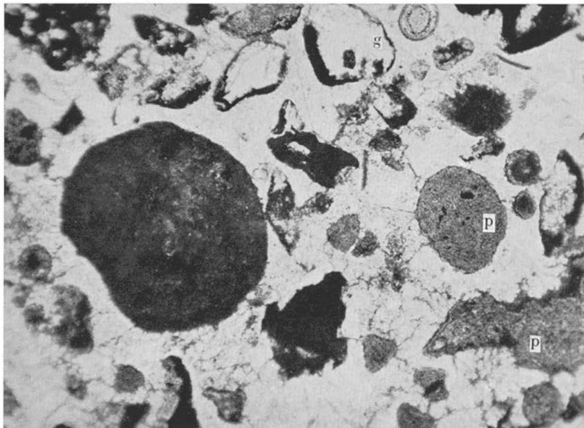
Fig. 78. Ceratopyge limestone. Pellets of phosphorite (p), grains of glauconite (g), and irregularly formed lumps of bitumen in matrix of fine-grained calcite. Lower Ordovician. Flagabro, Skåne. (Prep. 6316, photo 1298.) — 60×.
