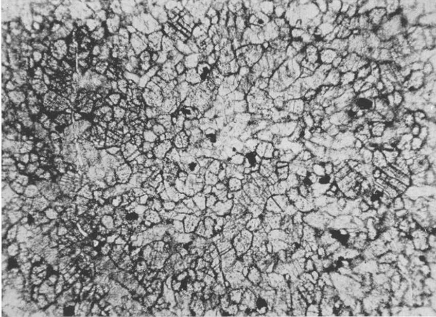
Fig. 1. Microcrystalline limestone, macroscopically dense. Planilimbata limestone. Ottenby, Öland. (Prep. 3007 b, photo. 1322.) — 60×.
