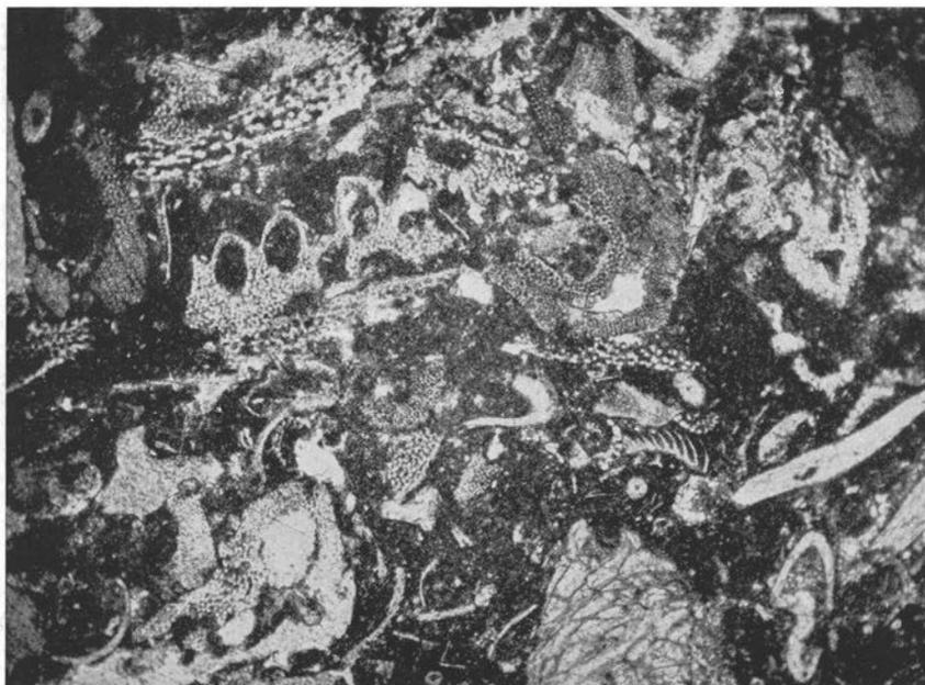
Fig. 150. Fragment limestone with pelmatozoans. Matrix argillaceous, microcrystalline calcite. Chasmops limestone, Middle Ordovician. N. Fredberga, Östergötland. (Prep. 7781, photo 1629.) — 20 ×.
