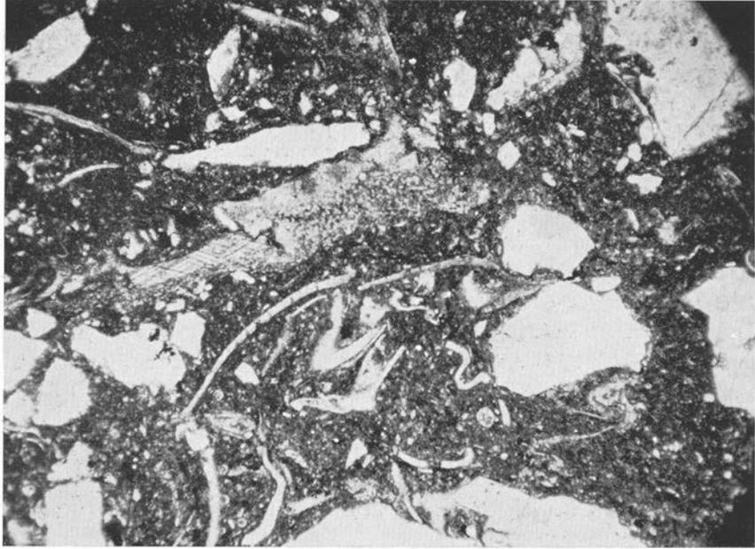
Fig. 154. Argillaceous microcoquina limestone, conglomeratic, with lumps of microcoquina limestone and granite shivers. Chasmops limestone (Loftarstone conglomerate), Middle Ordovician. Tandsbyn, Jämtland. (Prep. 5981, photo 1694.) — 20 ×.
