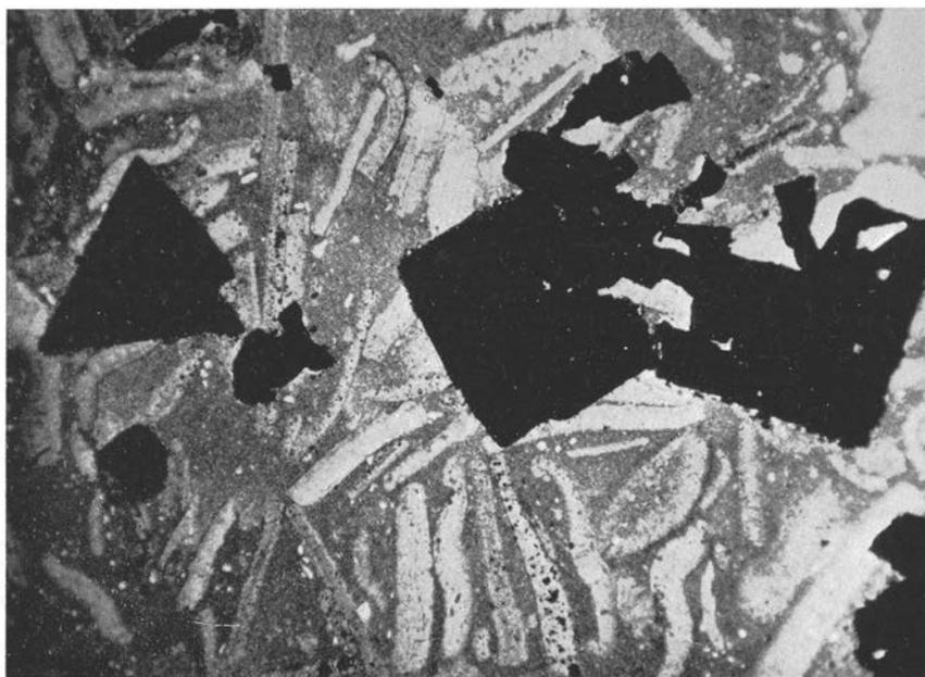
Fig. 13. Pyrite: crystals, aggregates, and dust. Fragment limestone. Lower Cambrian. Hardeberga, Skåne. (Prep. 8760, photo 1731.) — 20 $\times$ .
