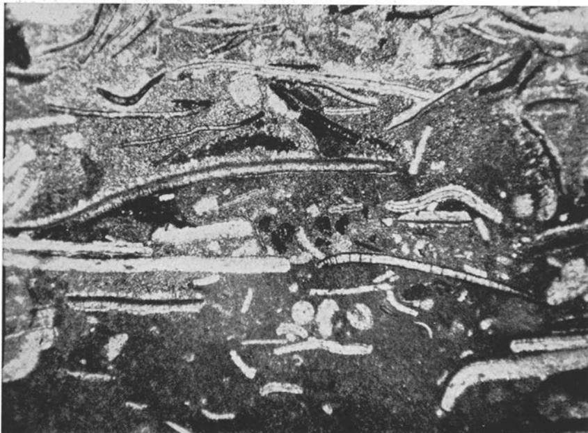
Fig. 58. Fragment limestone. Matrix microcrystalline, bituminous. Trilobite fragments and simple sponges (?). Middle Cambrian. Laesaa, Bornholm. (Prep. 8765a, photo 1753.) — 20×.
