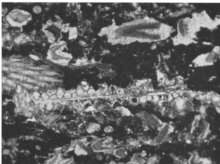
Fig. 191. Clink limestone ("Klingkalk") with dense, algal matrix and fragments of trilobites, crinoids, and bryozoans. Dalmanitina limestone, Upper Ordovician. Skattungbyn, Dalarna. (Prep. 6891, photo 1714.) — 20×.
