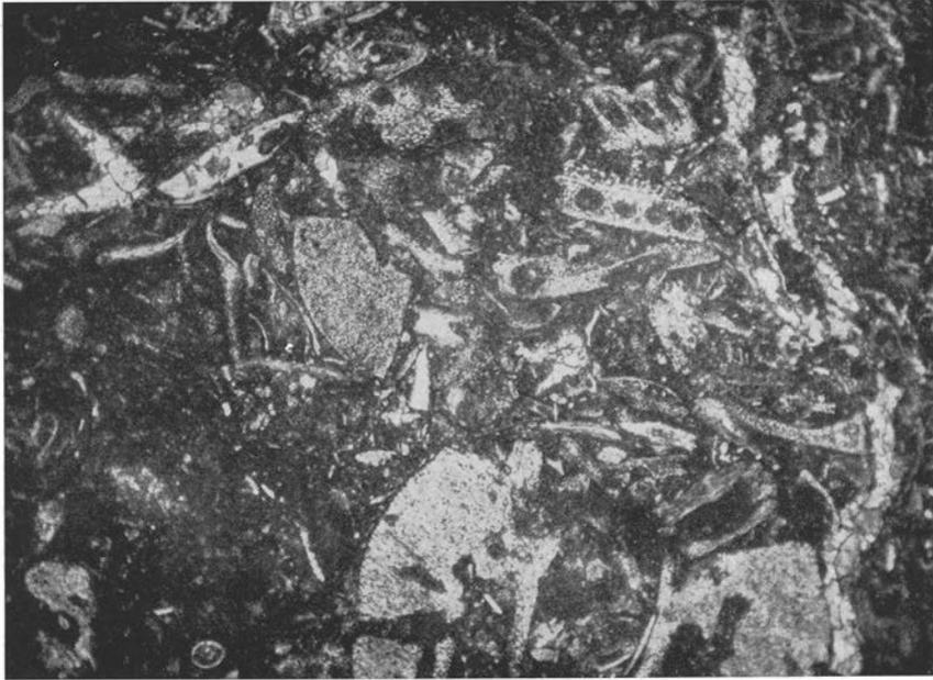
Fig. 141. Argillaceous fragment limestone with pelmatozoans. Crassicauda limestone ("Flagkalk"), Middle Ordovician. Fjäckå, Dalarna. (Prep. 7302, photo 1650.) — 20×.
