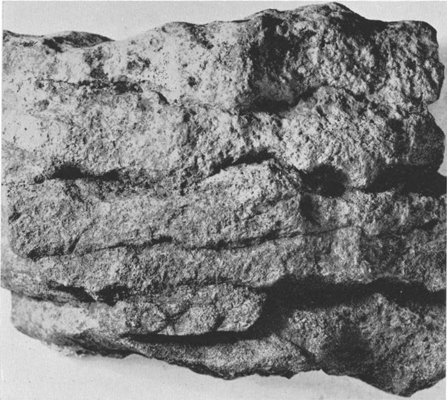
Fig. 98. Thin-bedded limestone. Asaphus limestone, Lower Ordovician. Resmo, Öland. (Photo 1495.) —  $\frac{1}{1}$ .
