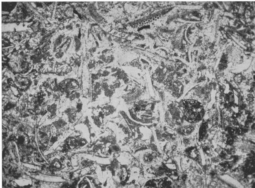
Fig. 140. Fragment limestone with microcoquina. Schroeteri limestone, Middle Ordovician. Kårgårde, Dalarna. (Prep. 8774, photo 1649.) — 20×.
