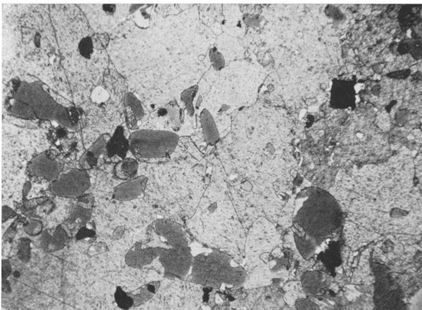
Fig. 90. Glauconitic limestone. Coarse-grained calcite with grains of glauconite, partly replaced by calcite. Planilimbata limestone, Lower Ordovician. Degerhamn, Öland. (Prep. 6524, photo 1789.) —  $30\times$ .
