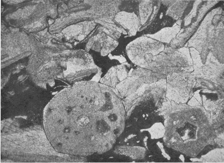
Fig. 99. Fragment limestone. Matrix partly coarse-crystalline calcite, partly argillaceous, cryptocrystalline hematite dust. Lower Asaphus limestone, Lower Ordovician. Ottenby, Öland. (Prep. 6628, photo 1639.) — 20×.
