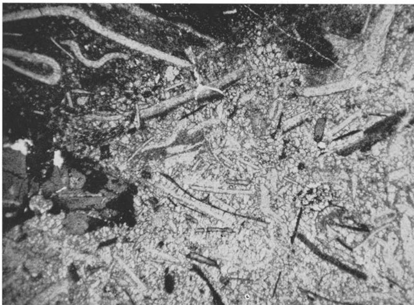
Fig. 55. Hyolithes limestone. Microcoquina with bituminous matrix and phosphatic nodules (left) and shells. Middle Cambrian. Andrarum. (Prep. 8764, photo 1737.) — 20×.
