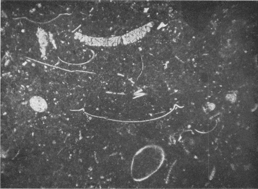
Fig. 143. Microcrystalline, flint-dense limestone. "Leversten". Schroeteri limestone, Middle Ordovician. Kinnekulle, Västergötland. (Prep. 3031, photo 1761.) — 20 ×.
