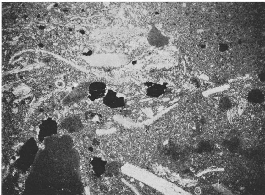
Fig. 116. Planilimbata limestone with recrystallized fragments, grains of glauconite (dark grey), and pyrite (black). Matrix even-grained, microcrystalline calcite and fragments. Lower Ordovician. Knivinge, Östergötland. (Prep. 7777, photo 1624.) — 20×.
