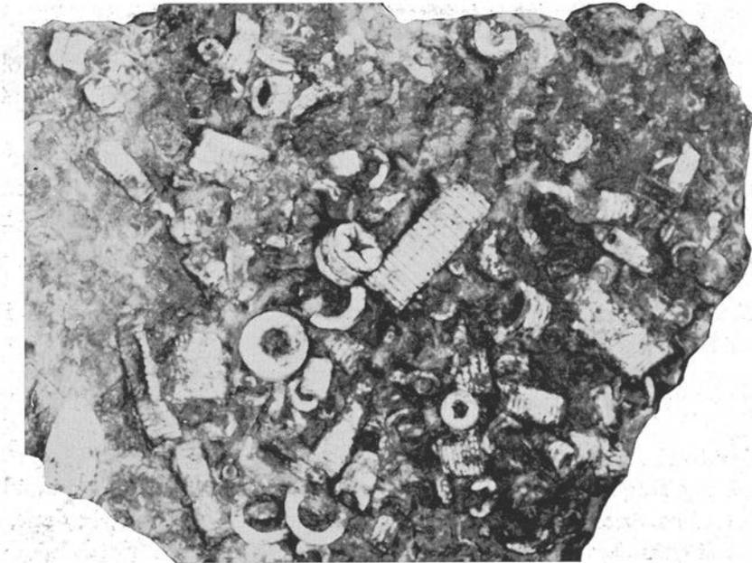
Fig. 186. Pelmatozoan limestone, thin-bedded, argillaceous. Chasmops limestone, Middle Ordovician. Amtjärn, Dalarna. (Photo 1792.) —  $\frac{1}{1}$ .
