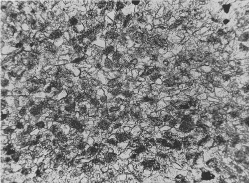
Fig. 177. Microcrystalline, arenaceous limestone with nodules (dark) of cryptocrystalline, algal calcite. Dalmanitina limestone, Upper Ordovician. Ålleberg, Västergötland. (Prep. 7795, photo 1716.) — 70 $\times$ .
