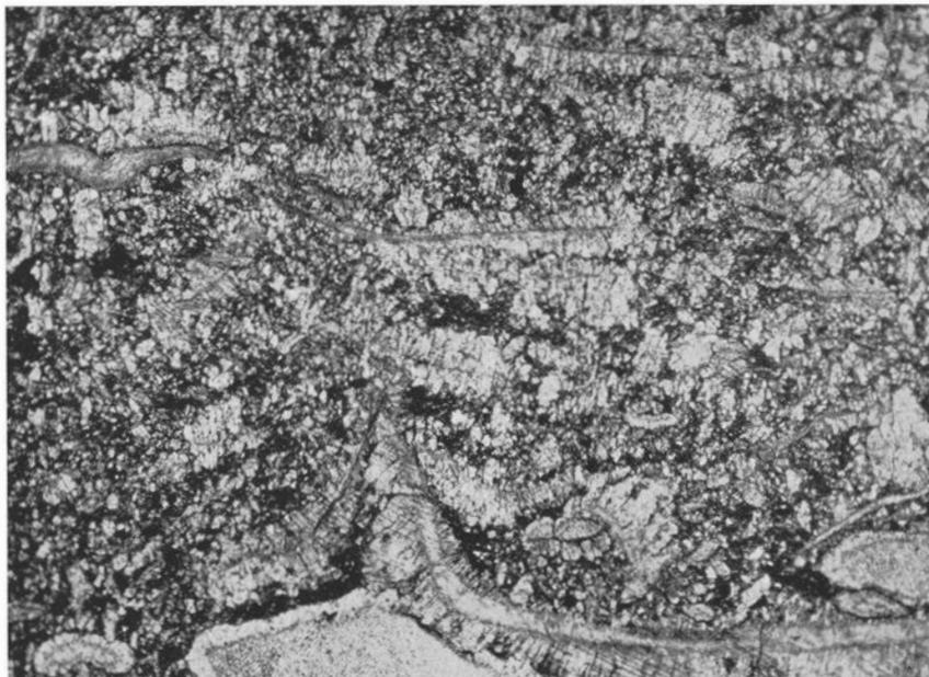
Fig. 3. Calcite crust on fossil fragments. Tretaspis limestone. Amtjärn. Dalarna. (Prep. 7213, photo 1653.) — 20 $\times$ .
