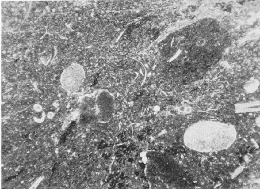
Fig. 145. Argillaceous, partly silicified limestone with cryptocrystalline, calcareous nodules. Chasmops limestone, Middle Ordovician. Öglunda, Västergötland. (Prep. 7254, photo 1709.) — 20×.
