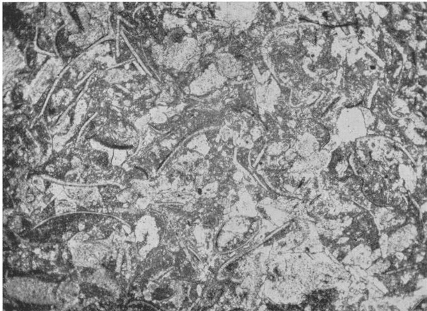
Fig. 180. Microcrystalline limestone with microcoquina. Dalmanitina limestone, Upper Ordovician. Gisseberg, Västergötland. (Prep. 7097, photo 1601.) — 20×.
