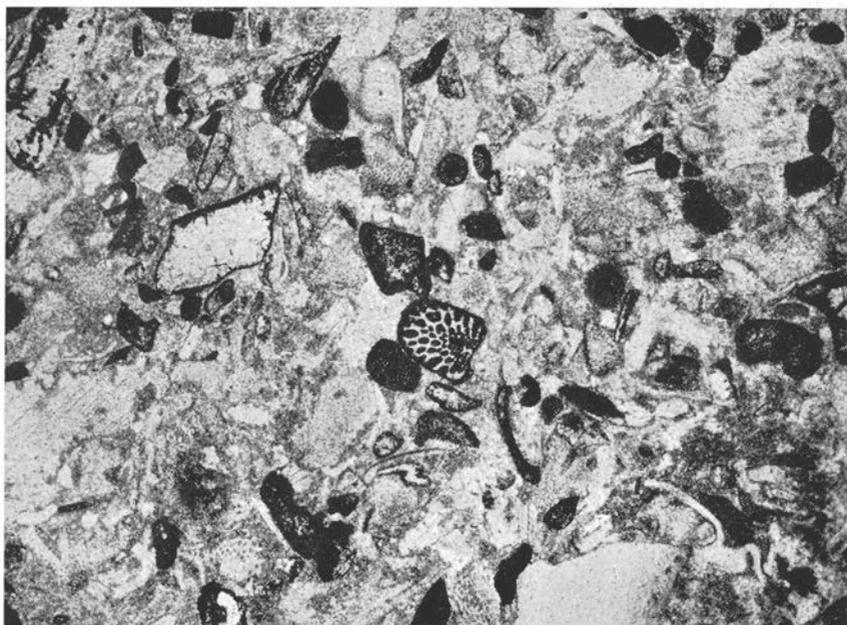
Fig. 125. *Expansus* limestone with irregularly pigmented fossil fragments. Lower Ordovician. Boda, Dalarna. (Prep. 7205, photo 1362.) — 20 $\times$ .
