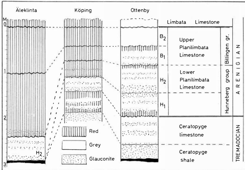
Fig. 93. Sections through the Ceratopyge and Planilimbata limestone of Öland (acc. to TJERNVIK 1956).
