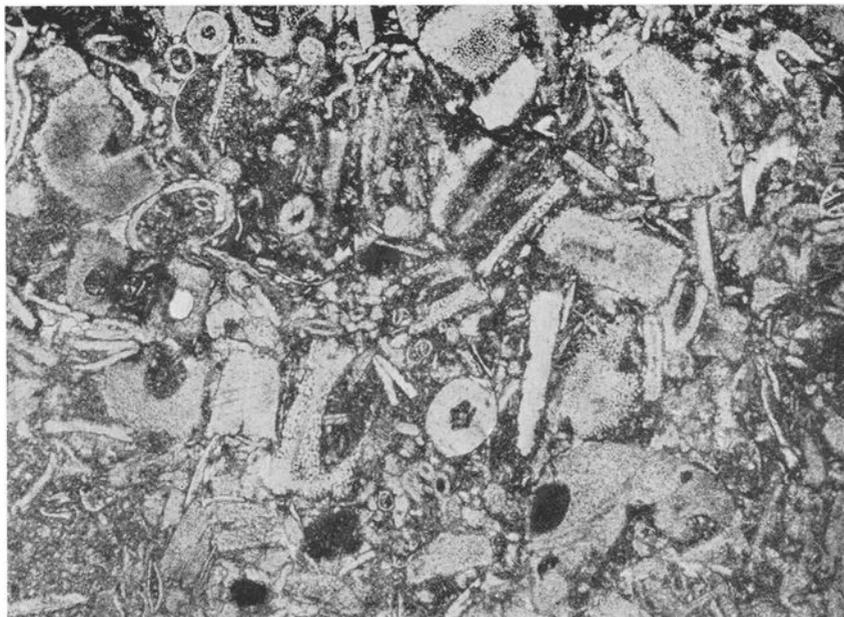
Fig. 96. Limbata limestone with pelmatozoans. Matrix: fine-grained fragments, microcrystalline calcite and hematite dust. Lower Ordovician. Resmo. Öland. (Prep. 6579, photo 1342.) — 20 × .
