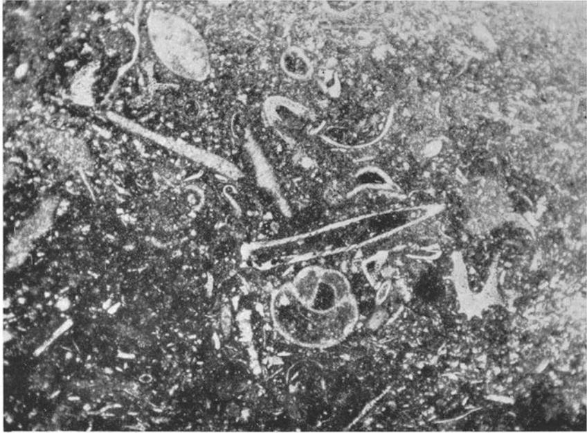
Fig. 131. *Platyurus* limestone. Microcoquina, hematite pigmented, with ostracods, gastropods and pelmatozoans. Lower Ordovician. Brunflo, Jämtland. (Prep. 7322, photo 1615.) — 20×.
