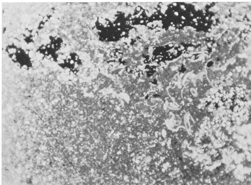
Fig. 168. Argillaceous, microcrystalline limestone with pyrite. Dalmanitina limestone, Upper Ordovician. Röstånga, Skåne. (Prep. 6884, photo 1718.) — 20 ×.
