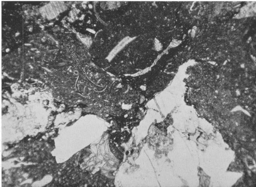
Fig. 155. Microcoquina limestone with redeposited material. Conglomeratic. Lumps of limestone (dark), shivers of granite (white). Chasmops limestone (Loftarstone conglomerate), Middle Ordovician. Tand, Jämtland. (Prep. 5987, photo 1759.) — 20 ×.
