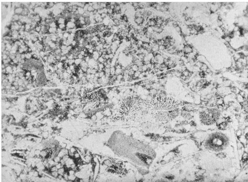
Fig. 138. Fragment limestone with pelmatozoans. Matrix of bitumen, argillaceous matter, and calcite grains. Orthoceras limestone, Lower Ordovician. Röstånga, Skåne. (Prep. 7103, photo 1692.) — 20×.
