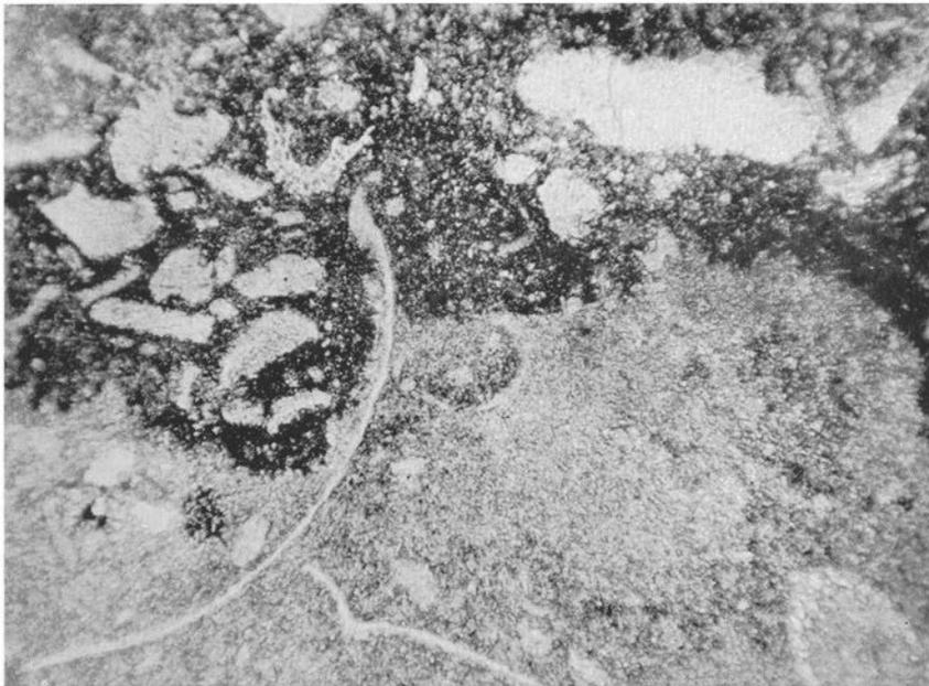
Fig. 17. Corrosion surface with protruding shell fragment. *Limbata* limestone, lower part yellow, upper red. Köping, Öland. (Prep. 6924, photo 1334.) —  $60\times$ .
