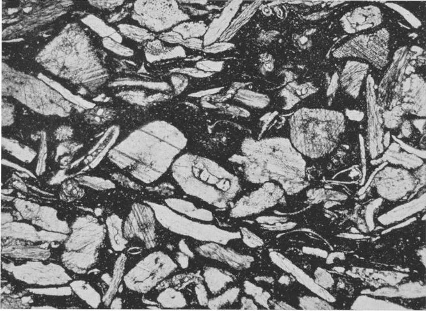
Fig. 152. Argillaceous and bituminous fragment limestone with redeposited material. Chasmops limestone, Middle Ordovician. Tand, Jämtland. (Prep. 694, photo 1367.) — 20 $\times$ .
