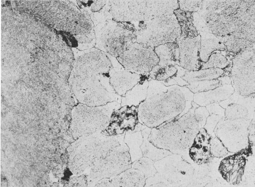
Fig. 24. Fragment limestone with grainy texture. Matrix strongly recrystallized. Slite group, Smöjen, Gotland. (Prep. 8216, photo 1561.) — 20 ×.
