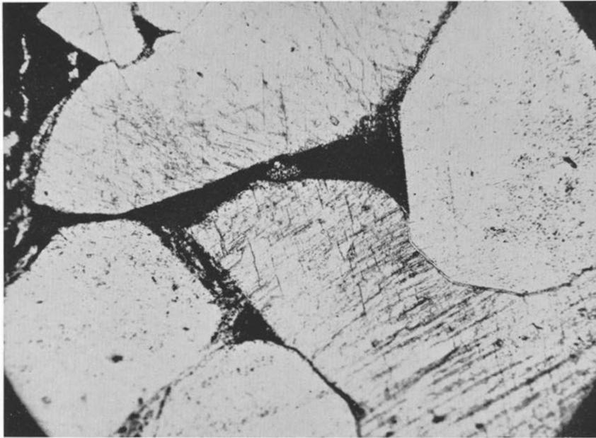
Fig. 30. Crystalline-granular texture. Matrix bituminous. Anthraconite. Lower Ordovician. Knivinge, Östergötland. (Prep. 7776, photo 1579.) — 60×.
