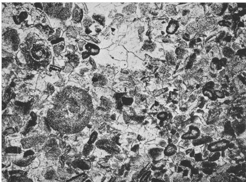
Fig. 102. Granular, glauconitic fragment limestone with crystalline matrix. Peripheral part of glauconite grains dark-pigmented. Lower Asaphus (*Expansus*) limestone, Lower Ordovician. Hälludden, Öland. (Prep. 6925, photo 1346.) — 20×.
