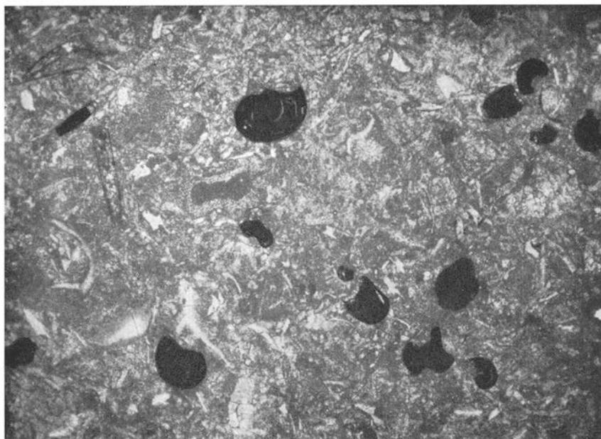
Fig. 126. *Microcoquina* limestone. Small gastropod shells filled with limonite. *Raniceps* limestone, Lower Ordovician. Åberga, Orsa, Dalarna. (Prep. 7827, photo 1647.) — 20 $\times$ .
