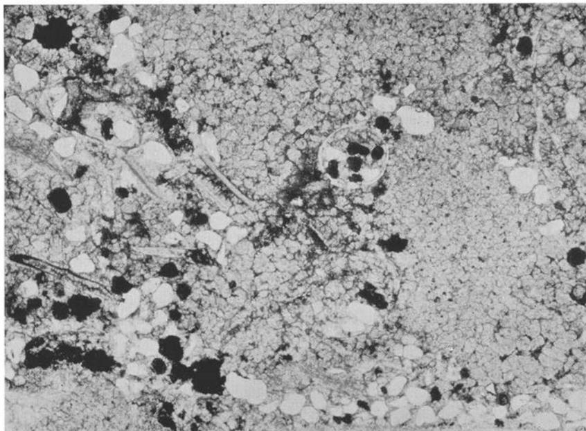
Fig. 59. Andrarum limestone. Microcrystalline, bituminous. Nodules without, matrix with grains of quartz and pyrite. Middle Cambrian. Laesaa, Bornholm. (Prep. 6563, photo 1467.) — 20×.
