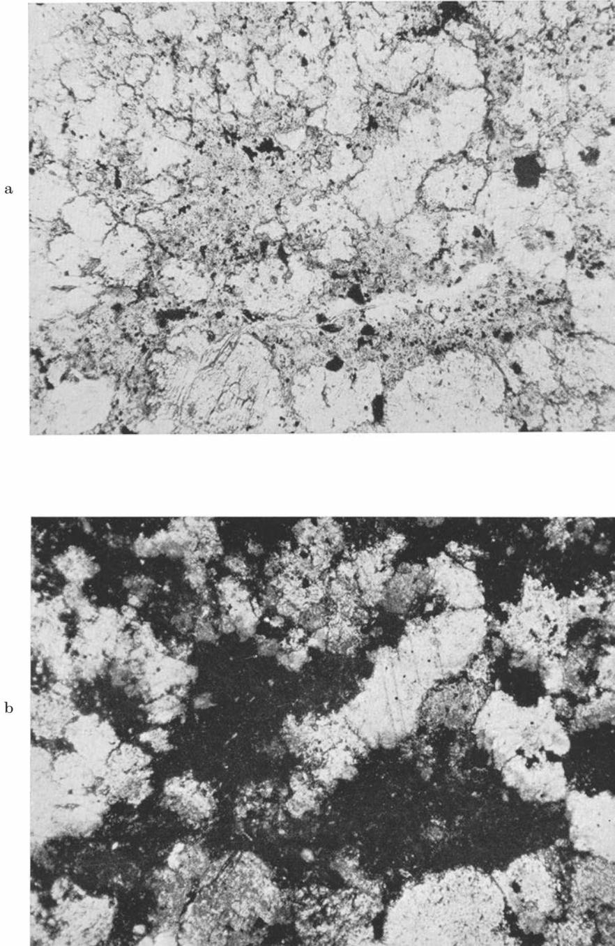
Fig. 165. Silicified limestone. Chasmops limestone, Middle Ordovician. Tommarp, Skåne.
