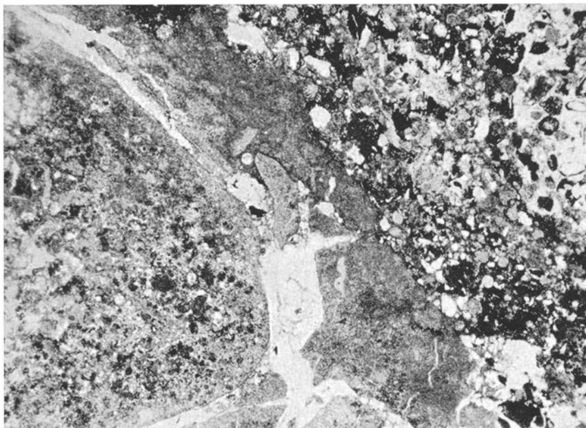
Fig. 12. Phosphatic nodule with crust of calcite and phosphorite. *Ceratopyge* limestone. Flagabro, Skåne. (Prep. 6316, photo 1292.) — 20 $\times$ .
