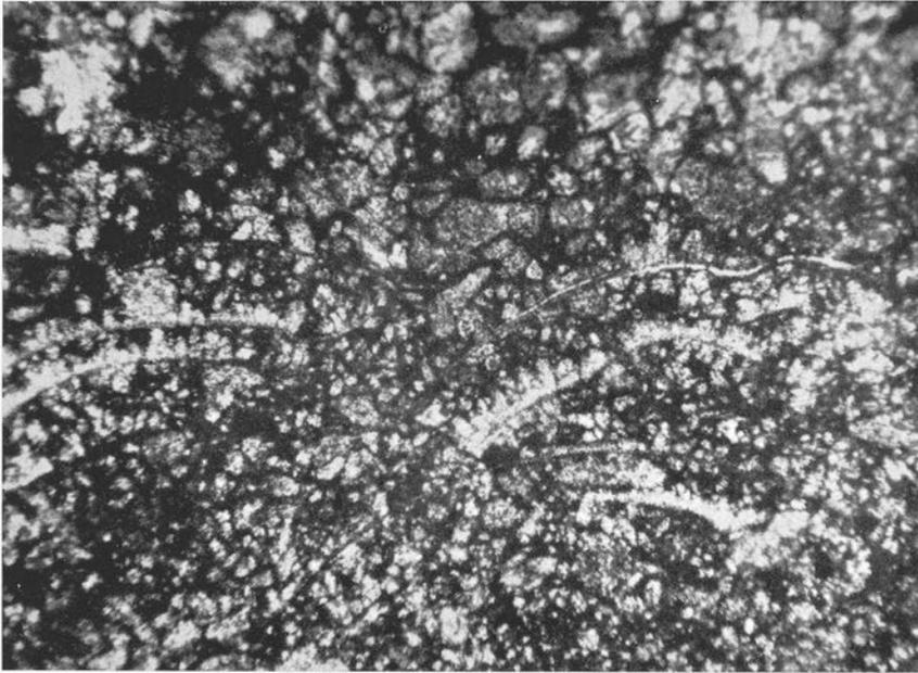
Fig. 72. Anthraconite, fine-grained, with radiating calcite crystals on fossil fragments. Upper Cambrian. Gudhem, Västergötland. (Prep. 6638, photo 1581.) —  $13\times$ .
