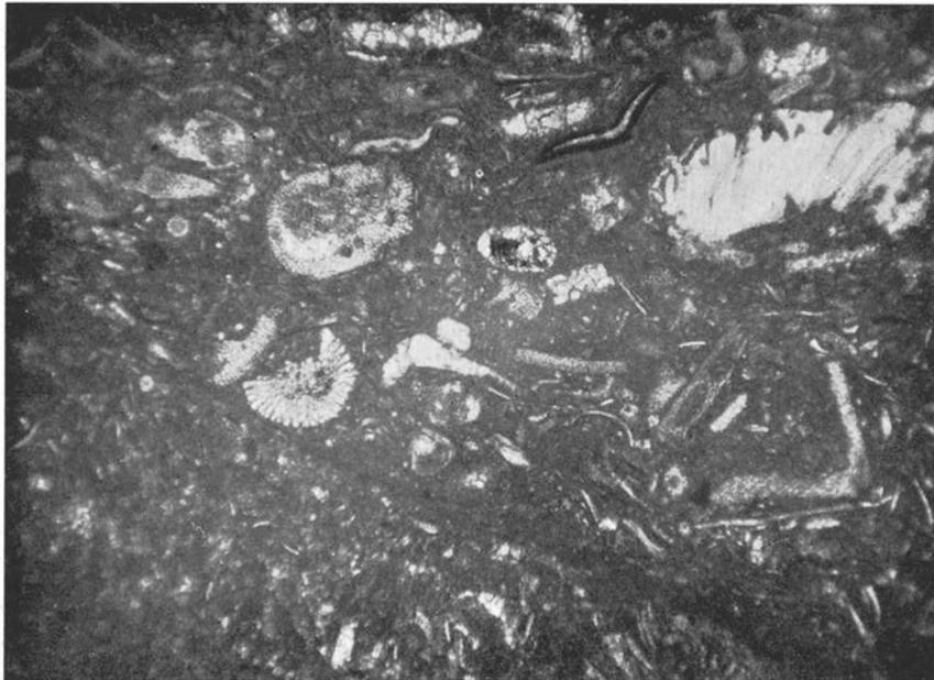
Fig. 142. Argillaceous microcoquina limestone. Ludibundus (Cystoidean) limestone, Middle Ordovician. Fjäckå, Dalarna. (Prep. 7321, photo 1764.) — 20×.
