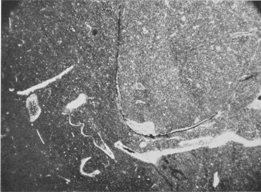
Fig. 163. Argillaceous, microcrystalline limestone (calcilutite). Bronni limestone, Middle Ordovician. Tommarp, Skåne. (Prep. 6539, photo 1699.) — 20 ×.
