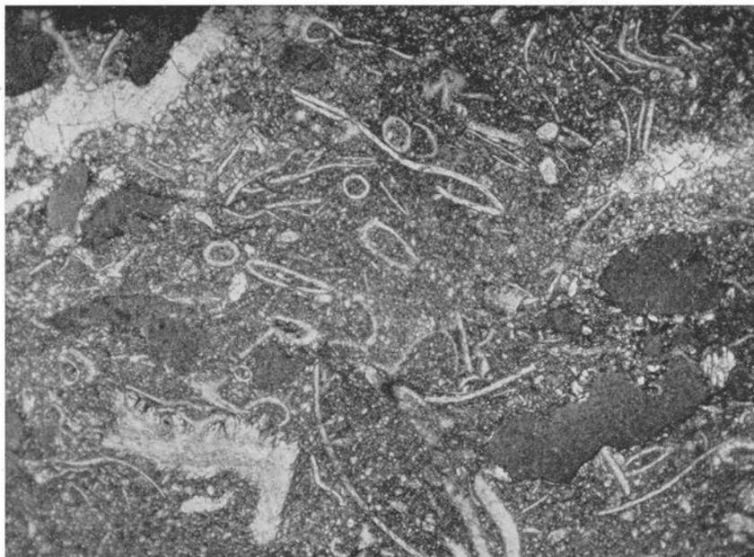
Fig. 120. Microcoquina limestone with glauconite grains. Planilimbata limestone, Lower Ordovician. Sjurberg, Dalarna. (Prep. 7211, photo 1646.) — 20 ×.
