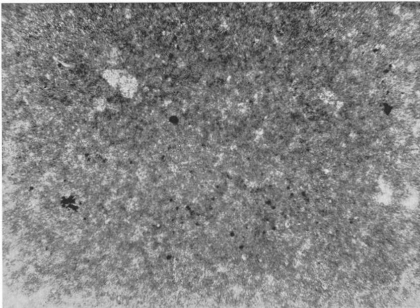
Fig. 185. Masur limestone, crypto- and microcrystalline, flocculent. Upper Ordovician. Fjäckå, Dalarna. (Prep. 7306, photo 1710.) —  $70\times$ .
