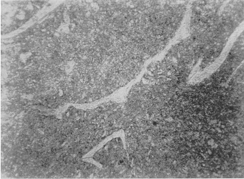
Fig. 97. Microcoquina limestone with strongly corroded fragments. Limbata limestone, Lower Ordovician. Bruddestad, Öland. (Prep. 6923, photo 1326.) — 60 ×.
