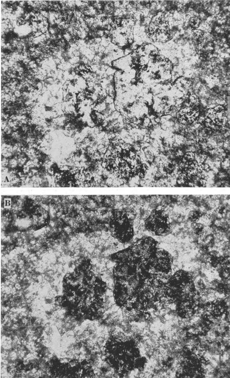
Fig. 183. Cordierite crystals in calcite aggregate. A) Nic. ||, B) Nic. +. Dalmanitina limestone, Upper Ordovician. Öglunda, Västergötland. (Prep. 7301, photo 1770 and 1771). — 90×.
