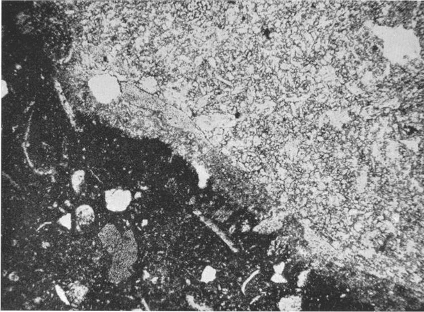
Fig. 117. Limbata limestone. Fragment limestone. Lower left: strongly pigmented, red and yellow, with grains of quartz (white) and glauconite (grey). Upper right: microcoquina. In the middle part band of glauconite. Lower Ordovician. Borghamn, Östergötland. (Prep. 7771a, photo 1628.) —  $33\times$ .
