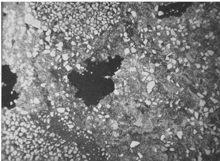
Fig. 42. Arenaceous, phosphoritic limestone. Lower left: phosphatic nodule filled with quartz. Black parts pyrite. Lower Cambrian. Hardeberga, Skåne.
