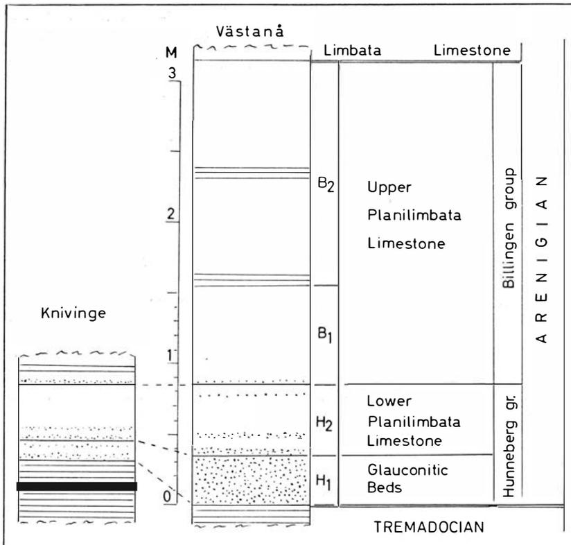
Fig. 115. Section through the Planilimbata limestone of Östergötland (acc. to TJERNVIK 1955).
