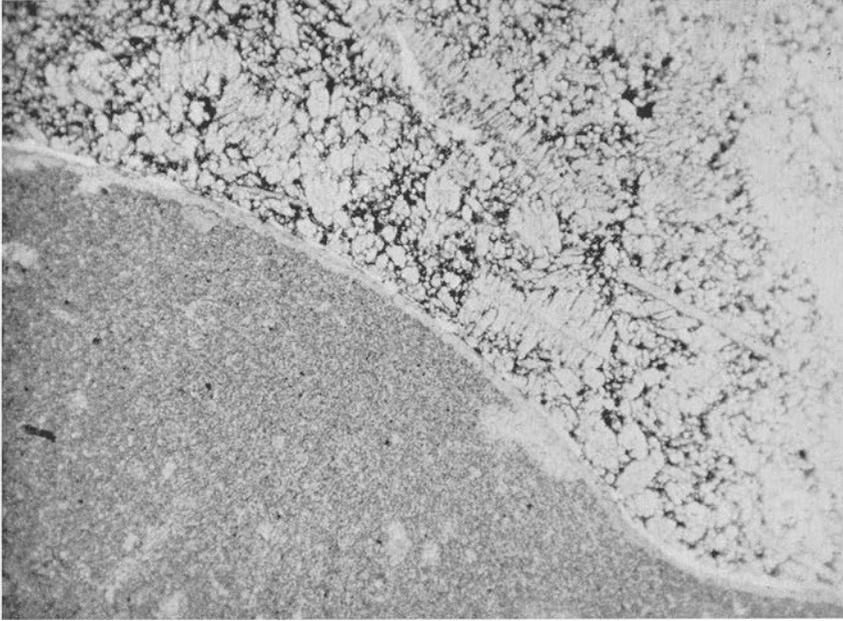
Fig. 52. Exsulans limestone. Lower part dense, dark, upper part light, recrystallized fragment limestone. At the boundary a trilobite carapace. Middle Cambrian. Brantevik, Skåne. (Prep. 7821, photo 1726.) — 20×.
