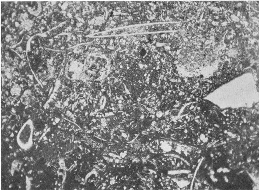
Fig. 144. Microcoquina limestone. "Leversten". Schroeteri limestone, Middle Ordovician. Öglunda, Västergötland. (Prep. 8776, photo 1612.) — 20 ×.
