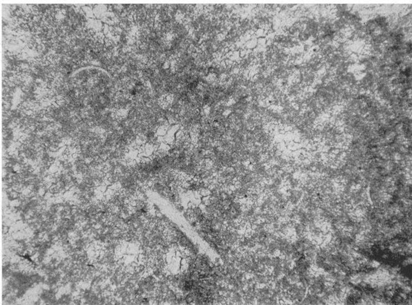
Fig. 170. Masur limestone. Flocky, partly cryptocrystalline, partly microcrystalline. Upper Ordovician. Erratic block. Brunby, Öland. (Prep. 6526, photo 1766.) — 20 ×.
