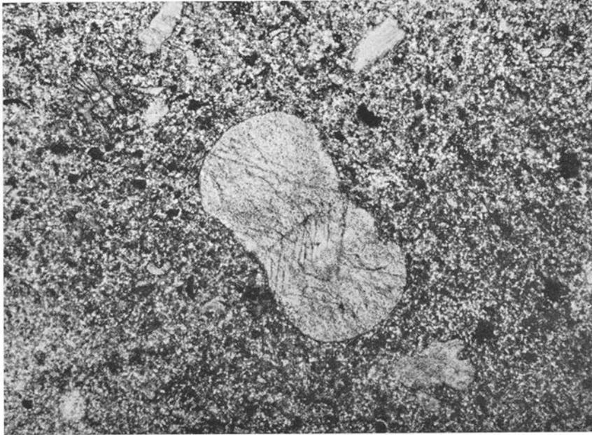
Fig. 161. Argillaceous, microcrystalline limestone (calcilutite) with pelmatozoan fragments. Macrourus limestone, Middle Ordovician. Ösby, Öland. (Prep. 3032, photo 1351.) — 20×.
