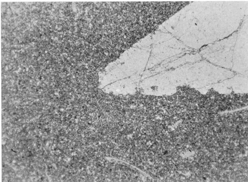
Fig. 167. Argillaceous, microcrystalline limestone with barytes crystal. Tretaspis limestone, Upper Ordovician. Jerrestad, Skåne. (Prep. 8904, photo 1719.) — 20 ×.
