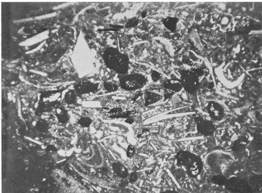
Fig. 159. Microcoquina limestone with limonite in porous fragments. *Crassicauda* limestone, Middle Ordovician. Stensåsa, Öland. (Prep. 6888, photo 1644.) — 20 ×.
