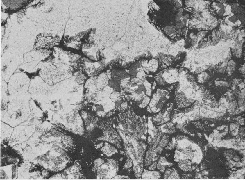
Fig. 91. Glauconitic limestone, hematite-pigmented, coarse-crystalline. Planilimbata limestone, Lower Ordovician. Mysinge hög. (Prep. 7140, photo 1400.) — 20 ×.
