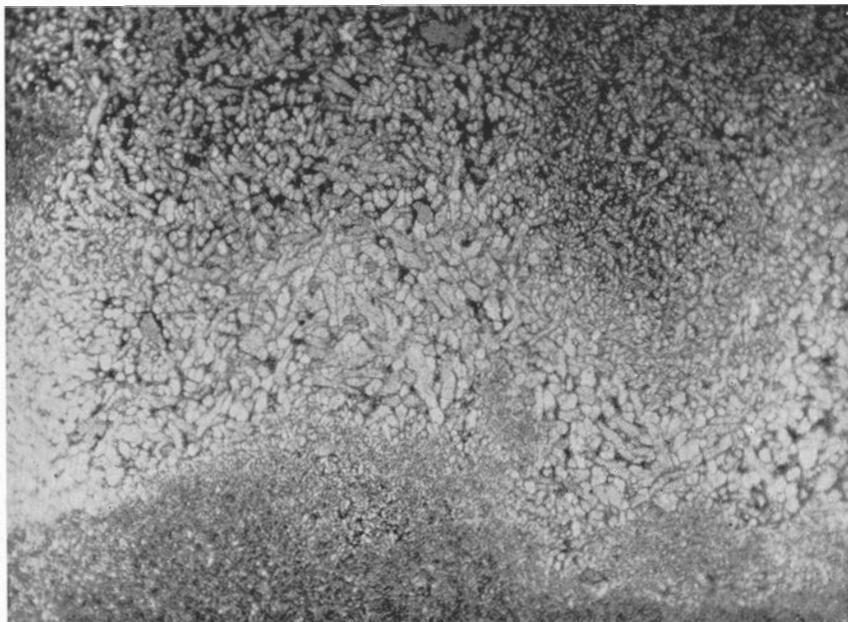
Fig. 4. Calcite grains in limonitic matrix. Planilimbata limestone. Skattungbyn, Dalarna. (Prep. 7825, photo 1689.) — 20 $\times$ .
