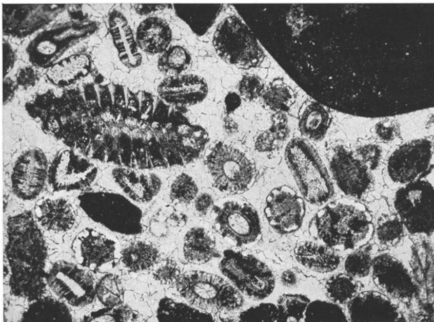
Fig. 173. Oolitic limestone with cryptocrystalline, algal nodules. Upper Ordovician. Erratic block. S. Fredberga, Östergötland. (Prep. 8798, photo 1630.) — 20×.
