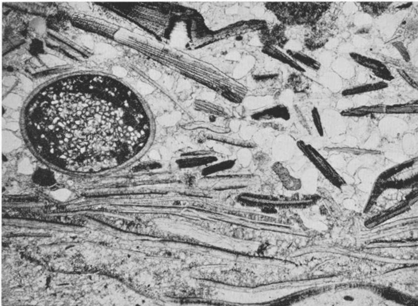
Fig. 65. Conglomeratic limestone. Matrix microcrystalline, with calcareous and phosphatic shell fragments, grains of quartz and glauconite, lumps of phosphorite. Granulata conglomerate, Middle Cambrian. Köping, Öland. (Prep. 7519, photo 1382.) — 20 × .
