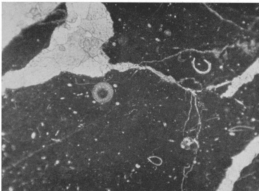
Fig. 149. Microcrystalline, flint-dense limestone with calcite veins. Chasmops limestone, Middle Ordovician. Kinnekulle, Västergötland. (Prep. 7093, photo 1763.) — 20 ×.
