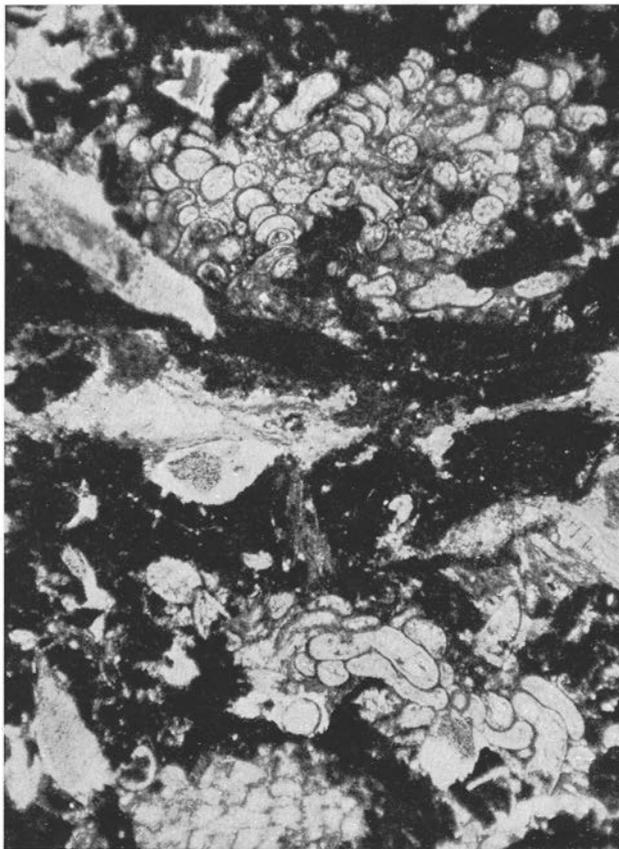
Fig. 193. Clink limestone. Dense, fibrous algal matrix (dark), and coarser algal threads and cells. Crinoidean and bryozoan fragments. Dalmanitina limestone, Upper Ordovician. Skattungbyn, Dalarna. (Prep. 6891, photo 1711.) — 20×.
