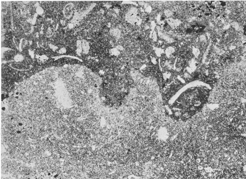
Fig. 147 b. Microcrystalline microcoquina limestone with corrosion surface. Chasmops limestone, Middle Ordovician. Skogastorp, Västergötland. (Prep. 7096, photo 1355.) — 20×.
