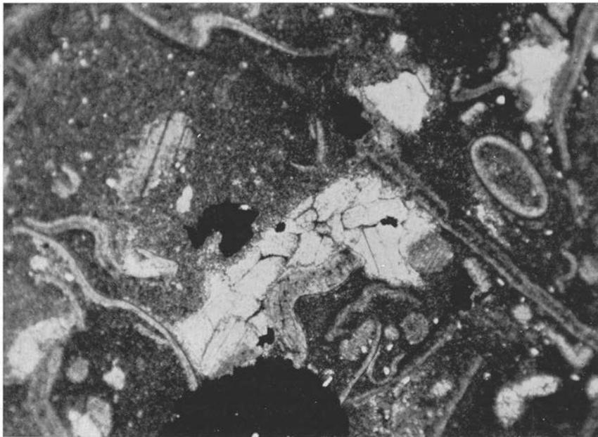
Fig. 50. Barytes (white), pyrite, and calcite (grey) in microcrystalline matrix. Fragment limestone. Middle Cambrian. Brantevik, Skåne. (Prep. 7787, photo 1740.) — 20×.
