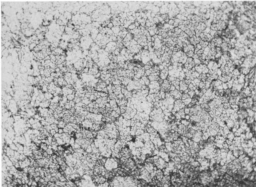
Fig. 132. *Platyurus* limestone. Completely recrystallized fragment limestone. Lower Ordovician. Andersön, Jämtland. (Prep. 7088, photo 1616.) — 20×.
