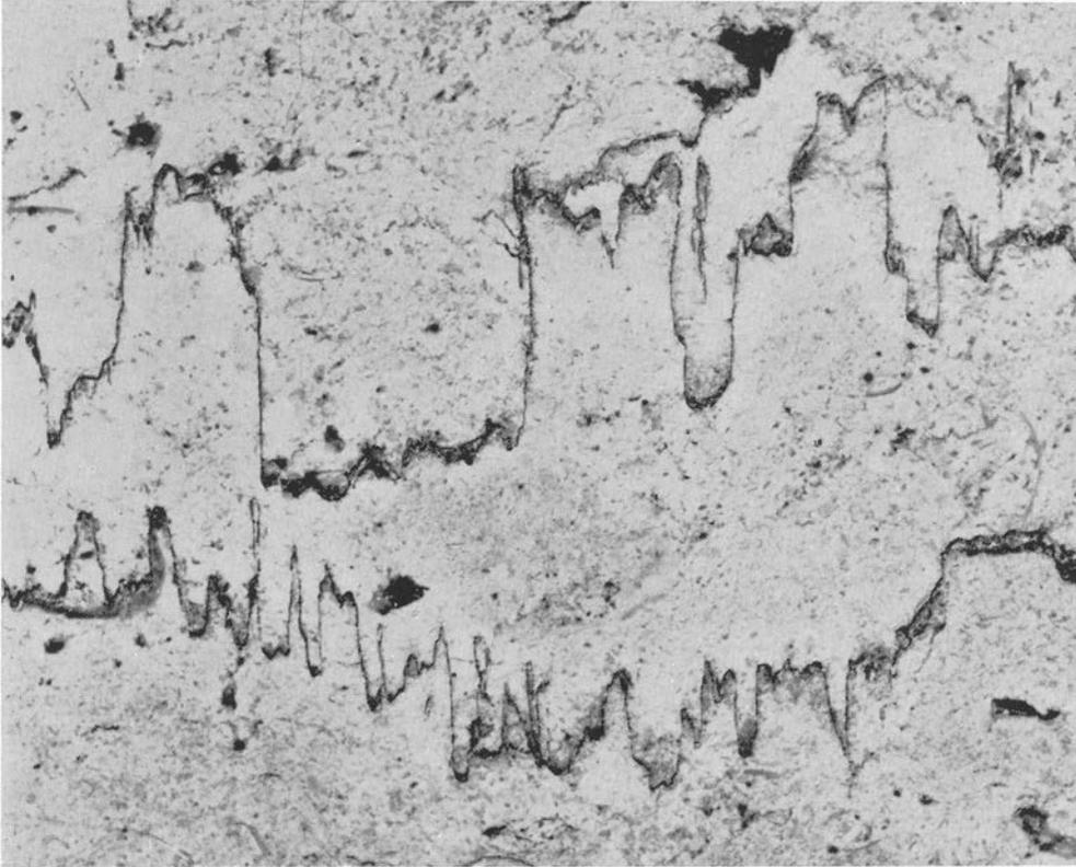
Fig. 20. Stylolites in pure, fine-grained fragment limestone. Slite group, Wenlockian. Storugns, Gotland.  $5.5\times$ . Foto. J. von Feilitzen.
