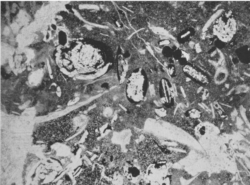
Fig. 164. Oolitic fragment limestone. Matrix of microcrystalline calcite with bitumen. Phosphorite (dark) and calcite partly replace the primary ooids. Bronni limestone, Middle Ordovician. Tommarp, Skåne. (Prep. 643, photo 1307.) — 20 ×.
