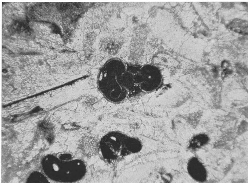
Fig. 128. Microcoquina limestone, strongly recrystallized. Platyrurus limestone, Lower Ordovician. Sollerön, Dalarna. (Prep. 7208, photo 1463.) — 60 $\times$ .
