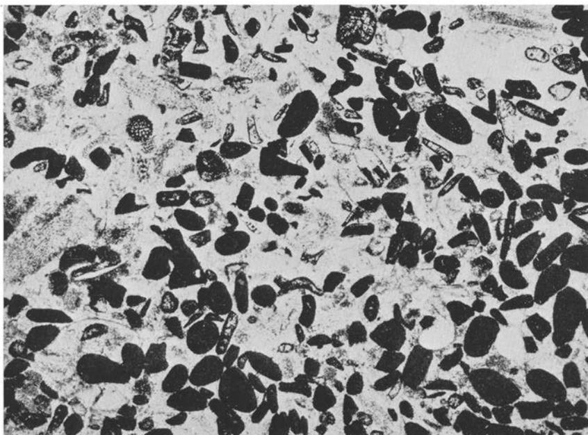
Fig. 124. Fragment limestone with ooids, pseudo-ooids and impregnations of limonite. Expansus limestone, Lower Ordovician. Utbyn, Rättvik, Dalarna. (Prep. 7198, photo 1361.) — 20×.
