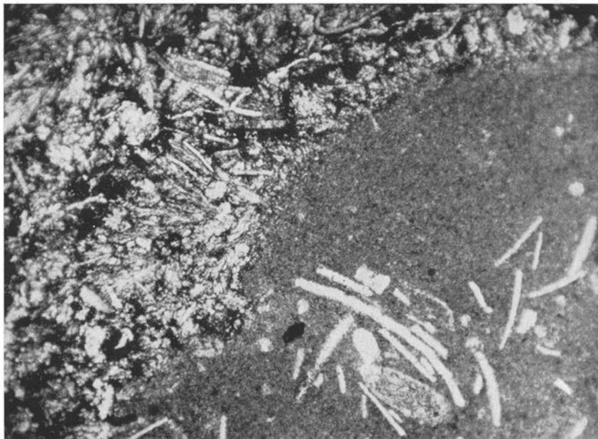
Fig. 53. Andrarum limestone. Dense, dark-grey and crystalline, black, bituminous fragment limestone. Middle Cambrian. Andrarum, Skåne. (Prep. 6561, photo 1725.) — 20×.
