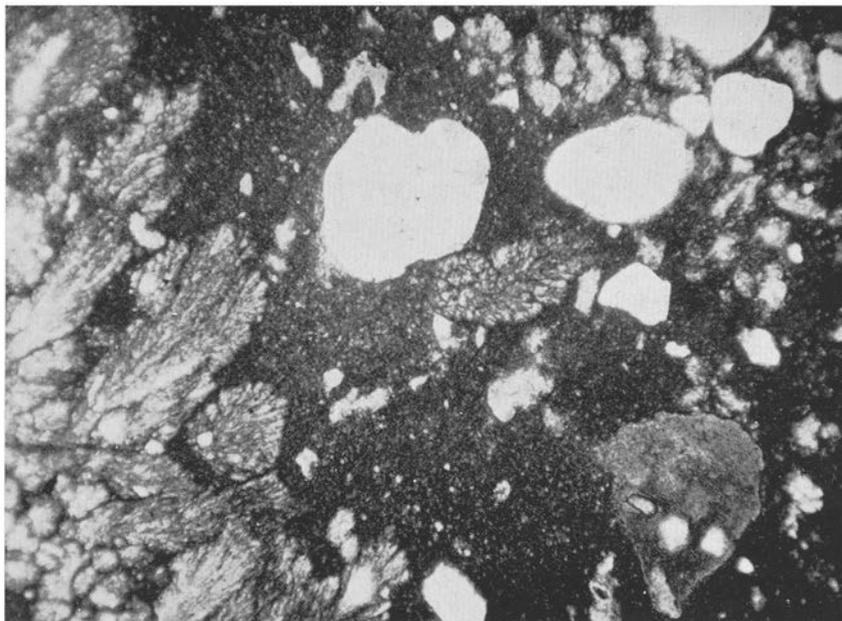
Fig. 38. Limestone with fibrous calcite crystals and quartz in argillaceous-bituminous matrix. Lower Cambrian. Luopaha, Lappland. (Prep. 2843, photo 1736.) —  $20\times$ .
