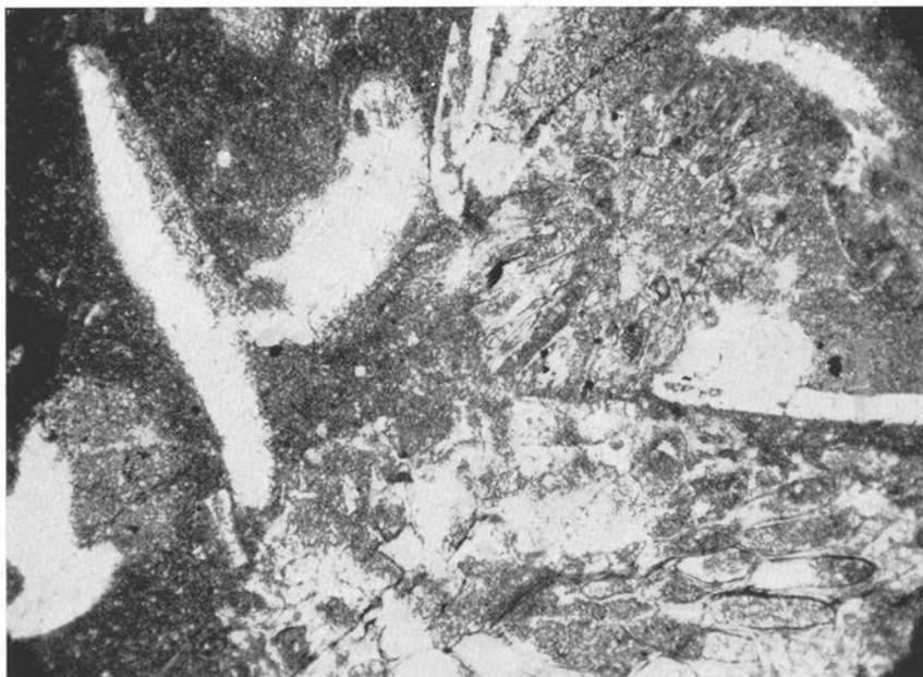
Fig. 157. Fragment limestone with bryozoans. Matrix argillaceous microcoquina and microcrystalline calcite. Middle Ordovician. Tand, Jämtland. (Prep. 7145, photo 1695.) — 20×.
