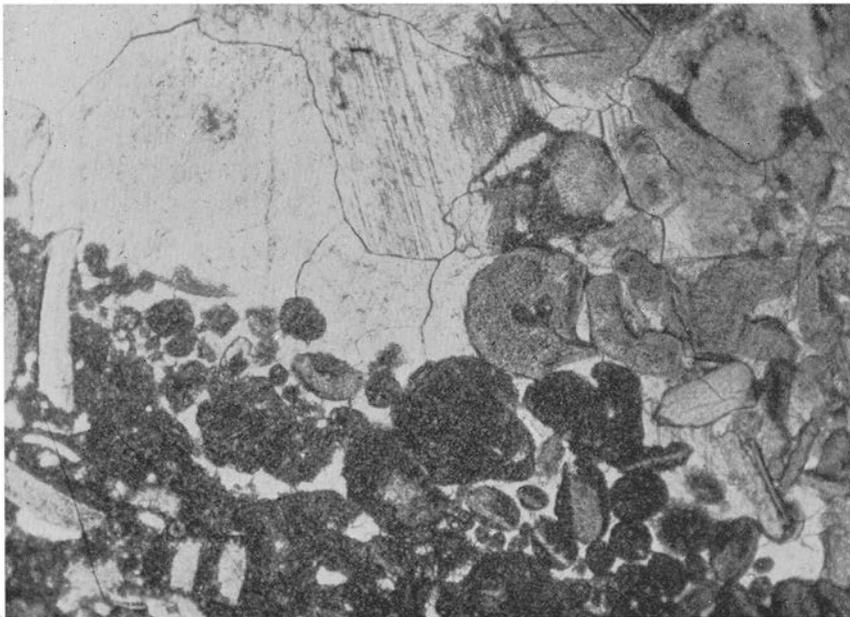
Fig. 119. Pelmatozoan limestone with crypto-crystalline (algal?) nodules. Asaphus limestone, Lower Ordovician. Borghamn, Östergötland. (Prep. 7774, photo 1687.) — 20 ×.
