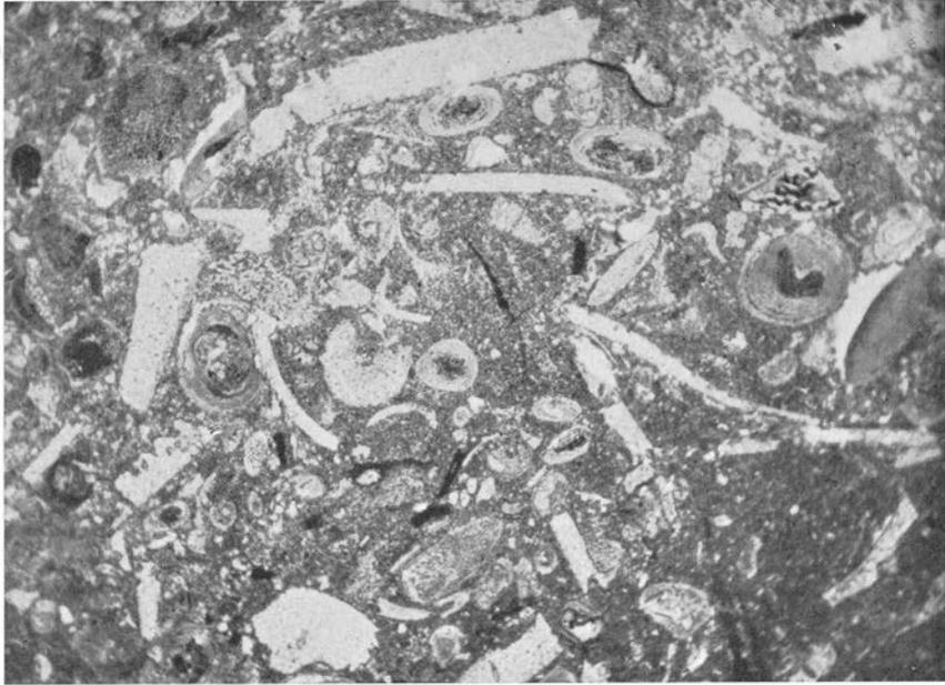
Fig. 146. Oolitic fragment limestone with microcoquina. Matrix of argillaceous, microcrystalline calcite. Echinospaerites limestone, Middle Ordovician. Ålleberg, Västergötland. (Prep. 8792, photo 1614.)
