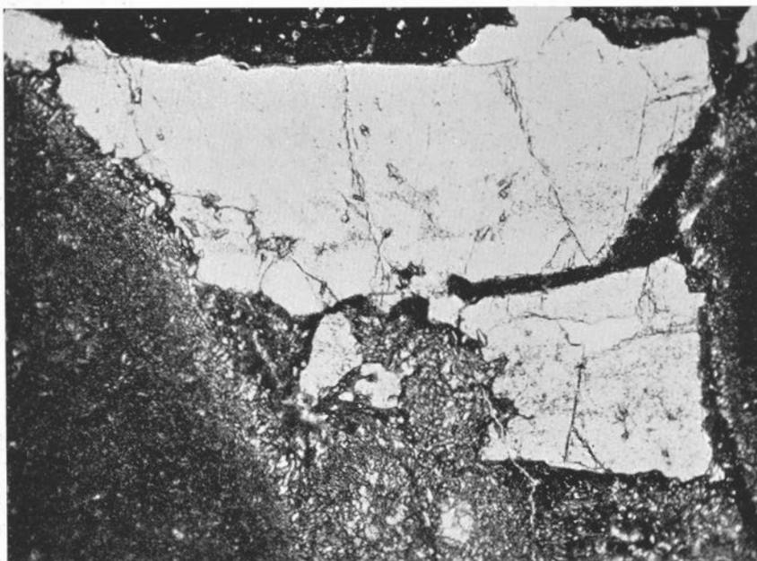
Fig. 109. Barytes crystals. Planilimbata limestone(?), Lower Ordovician. Hällekis, Västergötland. (Prep. 8767, photo 1591.) —  $20\times$ .
