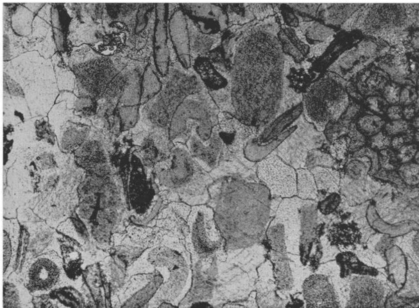
Fig. 8. Pure, crystalline fragment limestone. Slite group. Smöjen, Gotland. (Prep. 7406, photo 1524.) — 20×.
