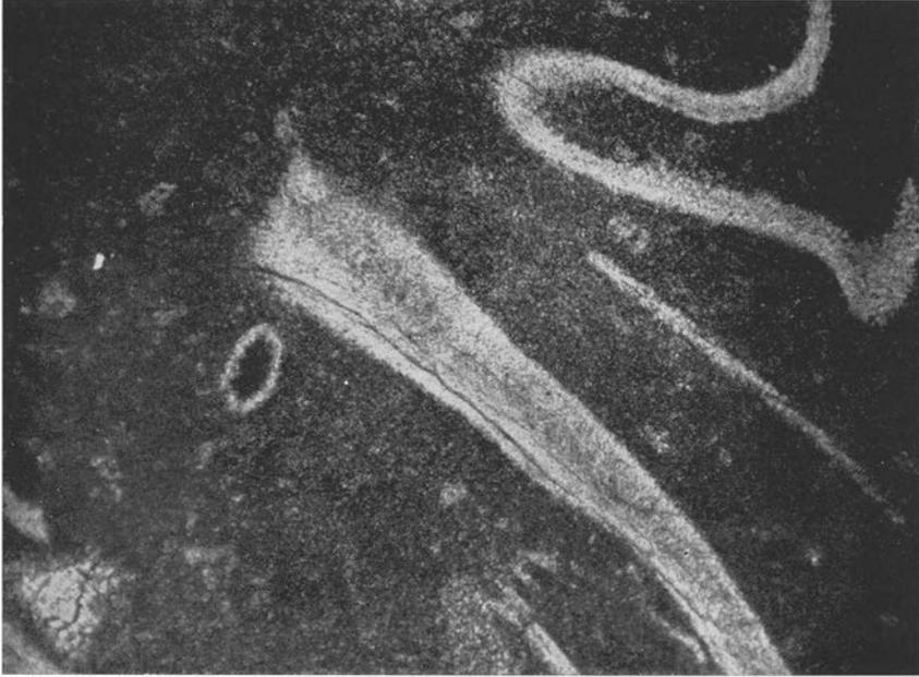
Fig. 82. Ceratopyge limestone. Matrix microcrystalline, evengrained. Recrystallized fragments of trilobites. Lower Ordovician, Flagabro, Skåne. (Prep. 6320, photo 1302.) — 20×.
