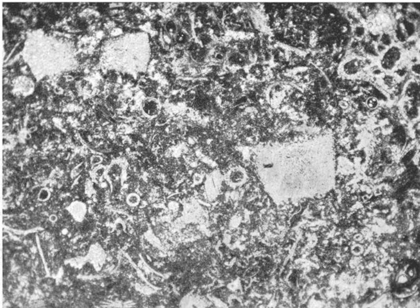
Fig. 162. Microcrystalline, partly silicified limestone with microcoquina. Macrourus limestone, Middle Ordovician. Hulterstad, Öland. (Prep. 7209, photo 1641.) — 20×.
