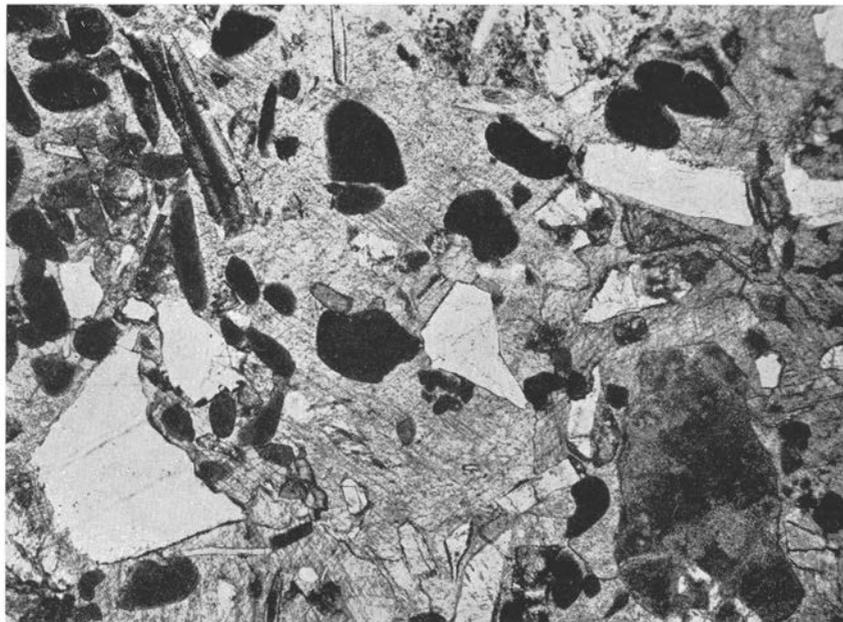
Fig. 86. Glauconitic limestone. Matrix of coarse-crystalline calcite, grains of glauconite (black) and phosphorite, splinters of granite. Lower Ordovician. Sjurberg, Dalarna. (Prep. 7548, photo 1359.) — 20 ×.
