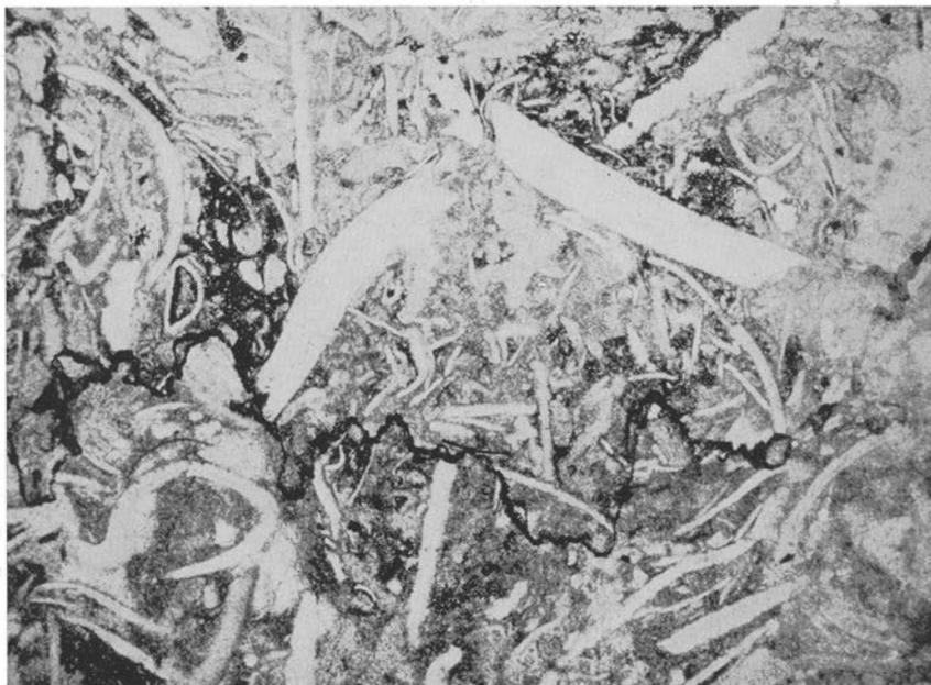
Fig. 137. Fragment limestone. Microcoquina recrystallized, grading over into matrix calcite. Limbata limestone, Lower Ordovician. Tommarp, Skåne. (Prep. 6541, photo 1305.) — 20×.
