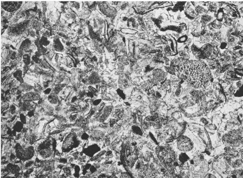
Fig. 25. Fine-grained fragment limestone. Asaphus limestone, Lower Ordovician. Hälludden, Öland. (Prep. 6925, photo 1409.) — 20 ×.
