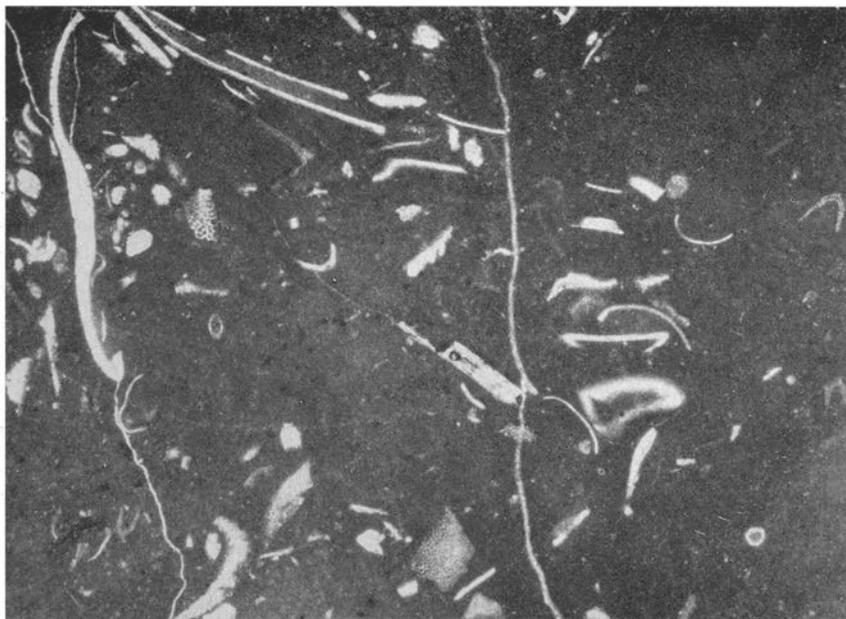
Fig. 174. Masur limestone, grumous, crypto- and microcrystalline. Tretaspis limestone, Upper Ordovician. Bestorp, Västergötland. (Prep. 2040, photo 1357.) — 20×.
