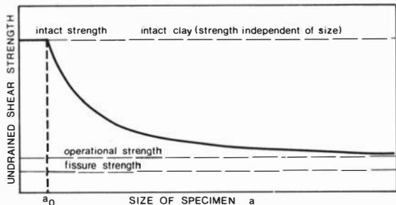
Fig. 4. Diagram of the strength-size relation (Lo, 1970).
