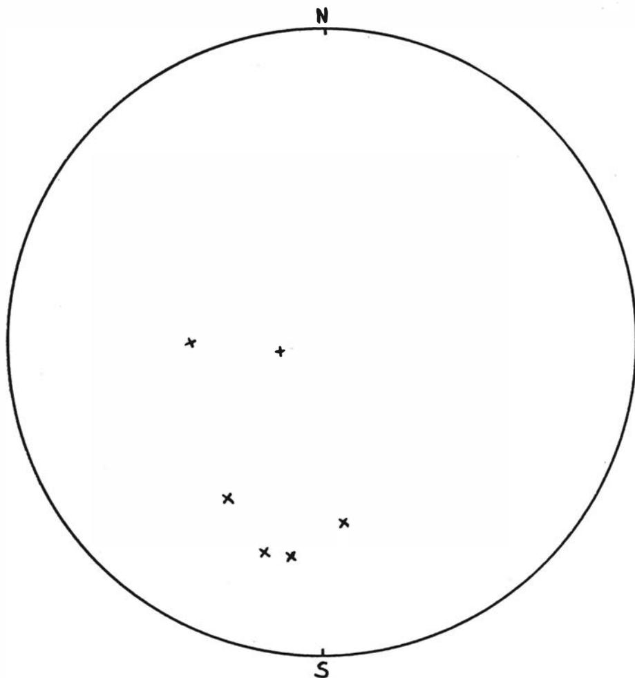
Fig. 5. A stereographic projection of the planes indicated in fig. 4. The crosses represent the poles of the planes. Two of the seven planes of fig. 4 coincide.
