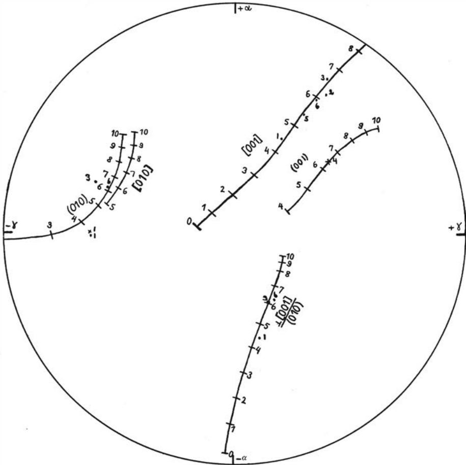
Fig. 16. A stereographic projection of the elements of twinning of the plagioclase in rock 15 at Bottorp. Dots indicate the axes of twinning, crosses the poles of the planes of twinning. The determinative curves are traced according to BEREK.
