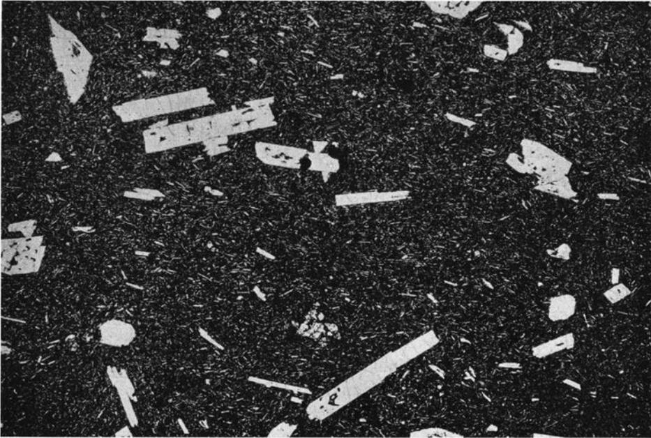
Fig. 27. Photomicrograph of basalt lava with phenocrysts of plagioclase, olivine, clinopyroxene and magnetite (No. 4 in Table IX and X). Tronador. Ord. light. Magnif.  $\times 10$ .
