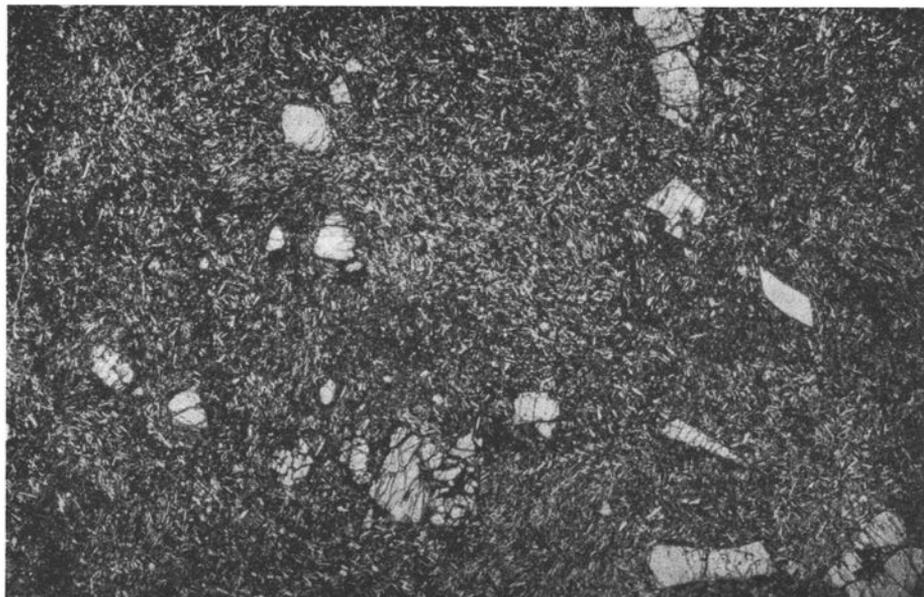
Fig. 36. Photomicrograph of intrusive olivine basalt with phenocrysts of olivine and plagioclase (very sparse). Peña de Columnas. Ord. light. Magnif.  $\times 11$ .
