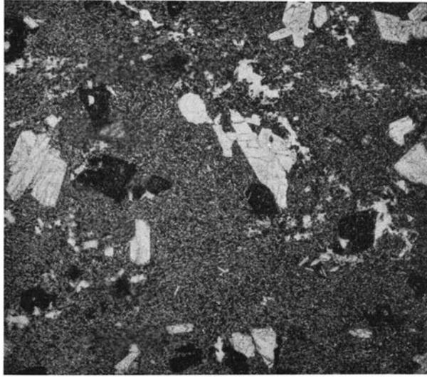
Fig. 33. Photomicrograph of olivine basalt with phenocrysts of plagioclase, olivine (opacitized) and diopside (No. 3 in Table XXVIII and XXIX). Calderón de Lavas. Ord. light. Magnif.  $\times 9$ .
