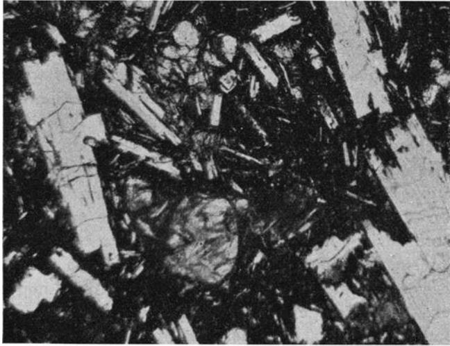
Fig. 26. Photomicrograph of basalt lava with phenocrysts of plagioclase and olivine (partly serpentinized; No. 8 in Table IV and V). Hill north of Paso Vuriloche. Ord. light. Magnif.  $\times 67$ .
