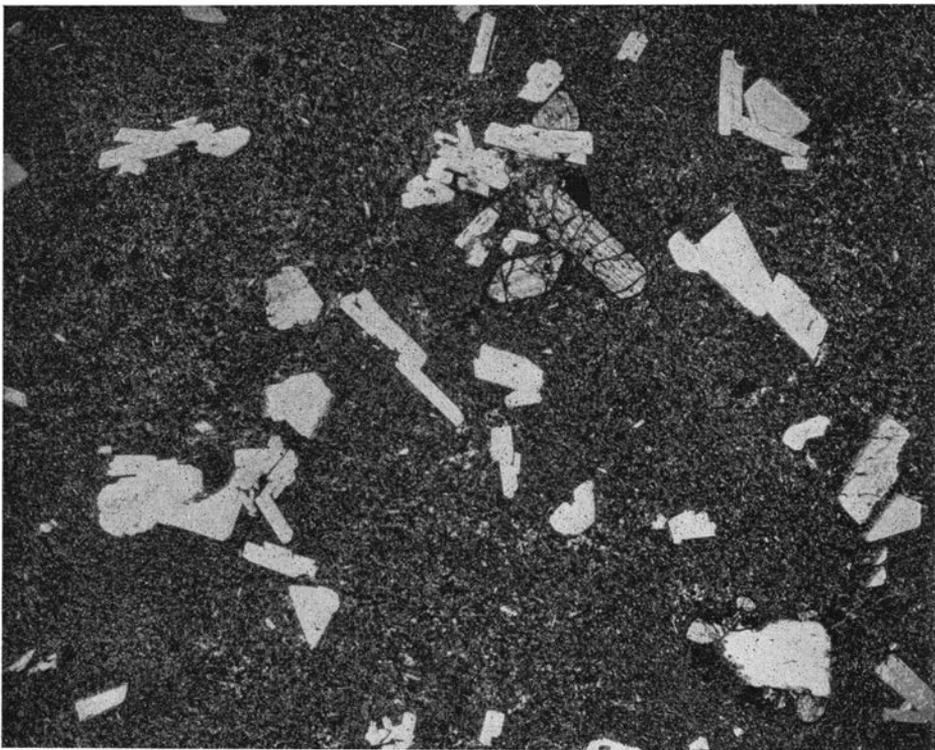
Fig. 29. Photomicrograph of pyroxene andesite with phenocrysts of plagioclase, orthopyroxene, clinopyroxene and magnetite (No. 1 in Table XIV and XV). Ventisquero Grande, Tronador. Ord. light. Magnif.  $\times 11$ .
