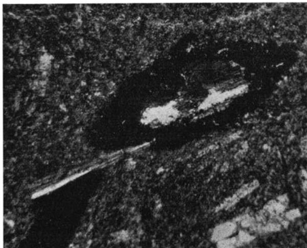
Fig. 30. Photomicrograph of hornblende dacite with phenocrysts of plagioclase, hornblende (largely resorbed), magnetite and apatite. Ventisquero Grande, Tronador. Ord. light. Magnif.  $\times 68$ .
