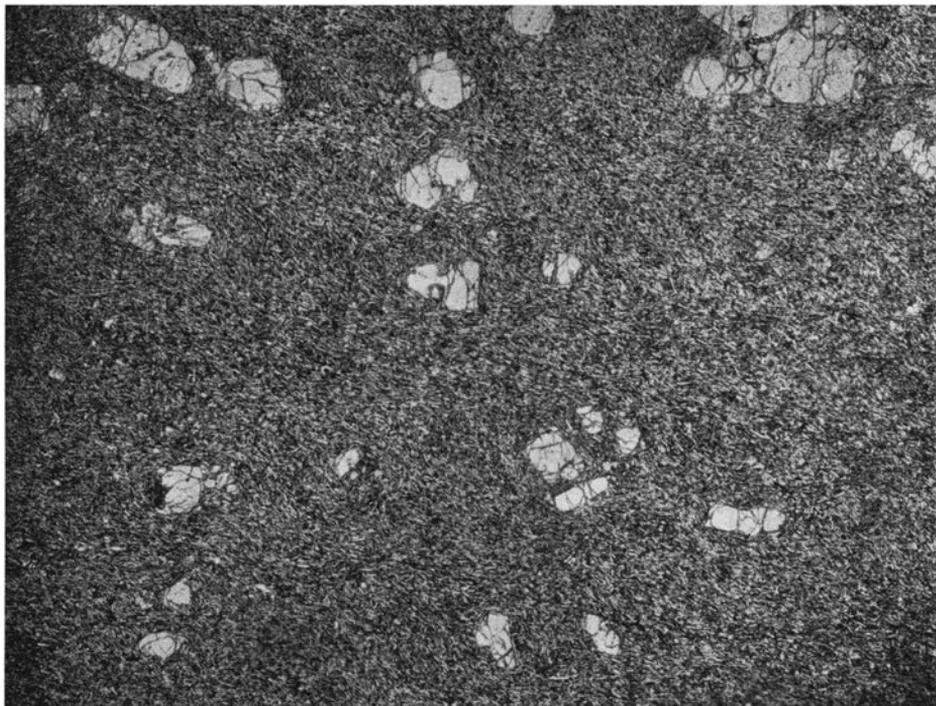
Fig. 32. Photomicrograph of olivine basalt with phenocrysts of olivine and diopside. East of Fraile. Ord. light. Magnif.  $\times 10$ .
