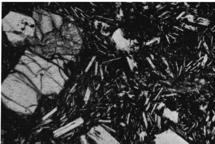
Fig. 25. Photomicrograph of basalt lava with phenocrysts of plagioclase, olivine and diopside (No. 3 in Table II and III). Tronador. Ord. light. Magnif.  $\times 68$ .
