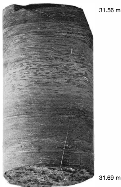
Fig. 3. Core section between 31.69–31.56 m showing speckled shale. Diplograptus multident Zone. Diameter of core 7 cm.
