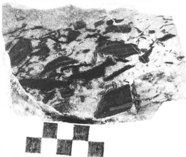
Fig. 37. Clay-pebble breccia in sandstone. Scale in centimetres. Polished hand specimen from an outcrop c. 3 km S of locality Mattarp 2 in Fig. 4.
