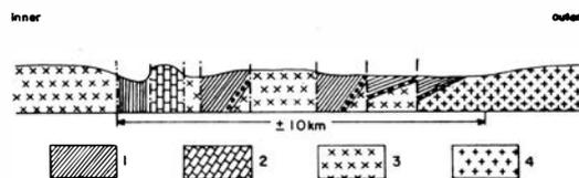
Fig. 6 — Schematic radical section across the Siljan ring. 1: Ordovician and Silurian. 2: Ordovician reef limestone. 3: Dala granite. 4: Earlier Precambrian.
