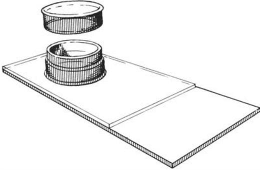
Text-fig. 2. Plastic box cemented to a glass slide which is glued on cardboard.
